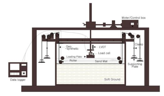
Figure 1. Model loading-experiment apparatus.
