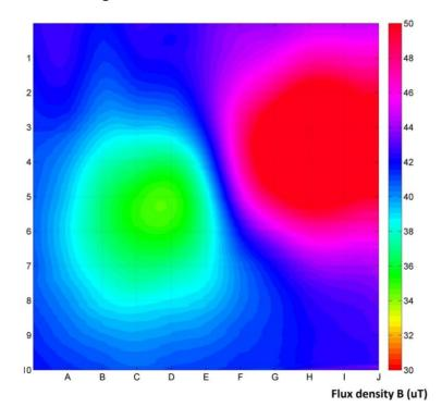
Distribution of flux density lines near a ferromagnetic object placed in the Earth's magnetic field is similar to a magnetic dipole field distribution. In particular, the magnetic flux density can be described as a dipole magnetic field characterized by a magnetic dipole moment  $\vec{m}$ . Induction of the magnetic field on the axis of the magnet, in a vacuum, at a distance *x* from its center is expressed by the formula:
