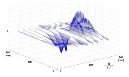
**Figure 4.** Visualization of the distribution of the magnetic induction vector absolute values, with the magnetic background intact. In addition to positive and negative disturbances, the Earth's magnetic field can be seen.
