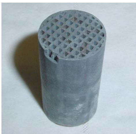
Figure 1. Siliconized silicon carbide (SiSiC) honeycomb structure used for testing.
