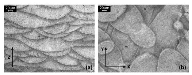
**Figure 7.** Optical microscope images after Weck's etching showing: (a) the presence of pores and at a higher magnification; (b) the shape of a melt pool with its contour.
