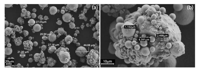
The numerous smallest particles, with mean diameters less than 10  $\mu$ m, tend to agglomerate on the surface of the bigger ones (Figure 3b), creating some clusters of about 60 to 80  $\mu$ m, and this could be detrimental for the final density of the DMLS parts, considering that the layer thickness employed in this research is of 30  $\mu$ m.
