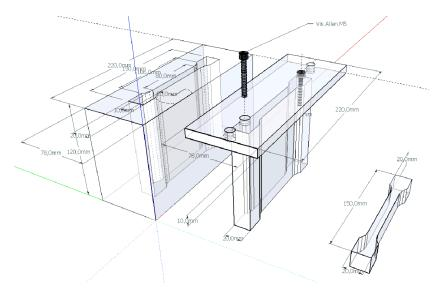
The  $\alpha$ -cellulose powder was pre-weighted and taken out of the climatic chamber in a closed container to maintain moisture content as much as possible. It was charged in the mold manually, as quickly as possible to prevent change of the moisture content, and great attention was paid at trying to get a homogeneous repartition.
