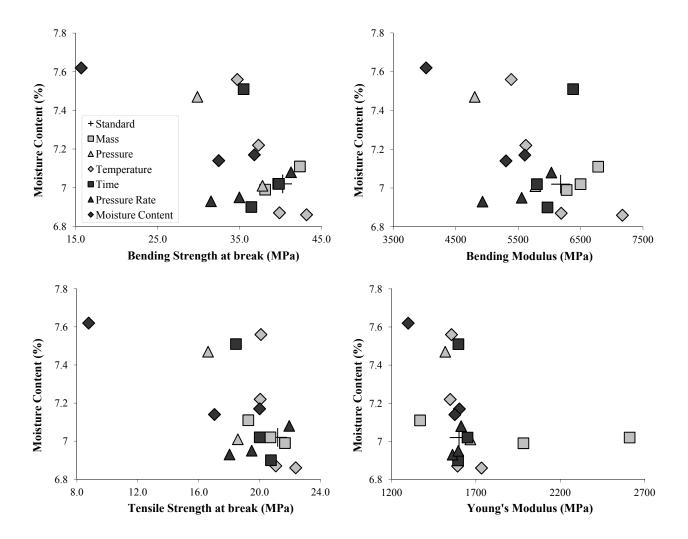
Figure 11 shows that specific gravity and moisture content were satisfactorily correlated, although the mechanical properties, representative of the bonding, could not be satisfactorily correlated to either specific gravity or moisture content, the mechanisms of bonding must therefore be complicated and imply several phenomena.
