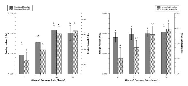
The Young's modulus was not impacted by the different conditions; these results are consistent with results obtained on pressure (Figure 5) and time (Figure 6) which had separately no impact on the Young's modulus.
