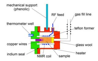
**Figure 4.** (Color on line) Schematic representation of the support structure and cooling path for the sample cell. The exterior copper can sits in a liquid helium bath that can be pumped to 1.4 K.
