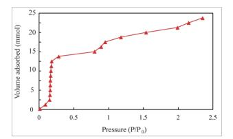
**Figure B1.** Adsorption isotherm for methane on zeolite-13X at 77 K.  $P_0 = 17$  mbar.
