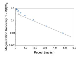
Understanding the origin of the two components for the relaxation is important for the analysis of the data. As an example we show in Figure A2 the relaxation observed for HD molecules at 5 K where two components are clearly visible. The ratio of the amplitudes can also be used to determine  $\mu$ , the ratio of the heat capacities of the baths.
