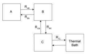
If these energy baths (A, B, C) can reach internal thermal equilibrium on a time scale smaller than that of the couplings between the baths, the observed overall relaxation will depend on the heat capacities of the individual baths. In particular, if as in Figure 1, the rate  $R_{BC}$  is the weakest (slowest) thermal link, the observed relaxation rate is given by
