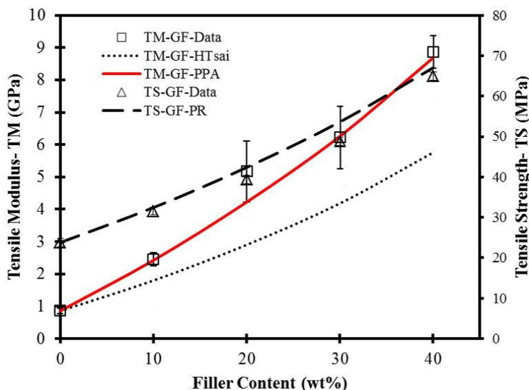
There is a near linearly increasing trend of tensile strength for composite. The strength increased to  $64.92 \pm 0.34$  MPa for GF-filled composites at the 40% GF loading level. Based on the statistical data
