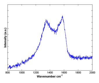
Figure 5. Raman spectrum of the products after treatment by HCl aqueous solutions.
