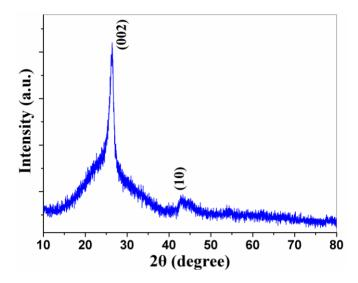
Figure 1. XRD pattern of the products after treatment with HCl aqueous solutions.
