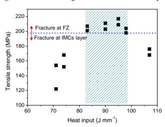
Figure 8. Tensile strength as a function of heat input.
