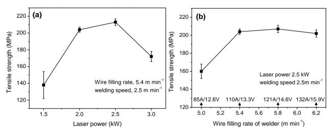
Figure 8 shows the relationship between heat input and tensile strength. It is found that the optimal range of heat input is 83-98 J mm<sup>-1</sup>. Within this range, all joints are stronger than 200 MPa and fracture in the FZ. Beyond this range, the joint are weaker than 200 MPa and fracture in the IMCs layer. When the heat input decreases to 71 J mm<sup>-1</sup>, the tensile strength reduces to the minimum, only 138 MPa.
