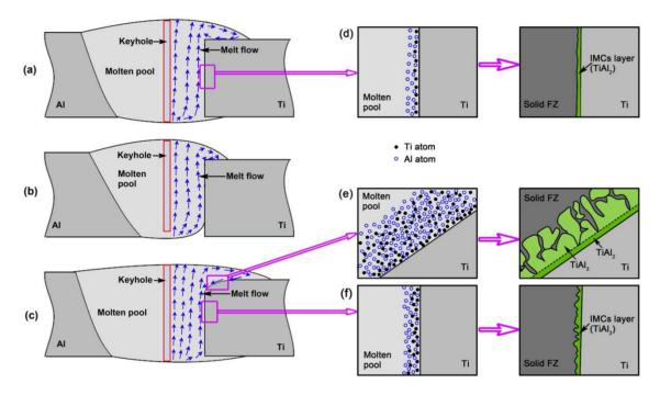
When laser power is inadequate, the laser keyhole obtained is shallow and the volume of melted metal in lower part is not enough because of insufficient heat input. As shown in Figure 11b, the melt flow is above the root of Ti6Al4V sheet, and do not full cover it. Lack of fusion then forms at the root. It also causes a too thin IMCs layer because of smaller amount of dissolved Ti atoms and faster solidification rate.
