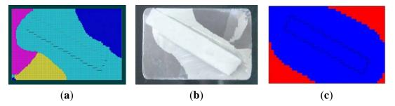
According to the definition above, IUZ has some features: (a) Stray grains of SX blades are mainly formed in IUZs; (b) The location and range of an IUZ are influenced and divided based on the temperature distribution; (c) IUZ often appears at some tips of the casting where heat dissipation is faster; (d) The analysis of IUZ is a convenient way to predict areas of the stray grain formation.
