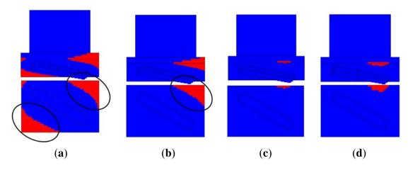
There are lots of factors influenced on the formation of IUZ, and withdrawal rate is an important one. The quick change of the cross-section area at the platform allowed more heat dissipation from the part below the platform, such as cooling zone or the water-cooled copper plate. Then at some edge or corner of the platform, the melt has a lower temperature than liquidus, but not turned to be solid, and the IUZs were formed.
