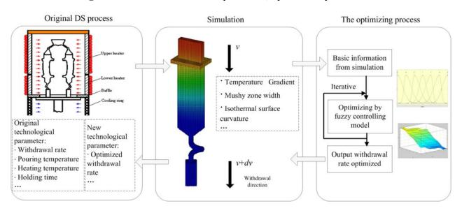
Figure2. The framework of DS processes, optimized by simulation.
