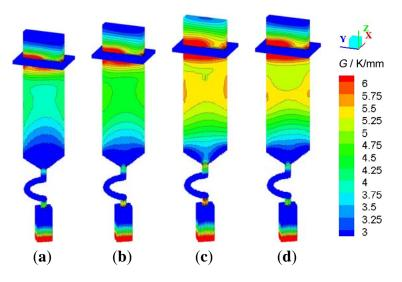
In conclusion, SG4 had a short solidification time than SG3, as shown in Figure 5, but its temperature gradients were higher than others. That is to say, at a proper time span, the DS process with an optimized withdrawal rate is benefit for improving microstructure and properties, and increasing productivity and yield rate of SX blades.
