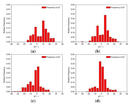
**Figure 13.** The frequency distributions of mushy zone width of the four simulation groups (a) SG1; (b) SG2; (c) SG3; (d) SG4.
