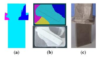
There are many reasons which caused stray grains, such as impurity of the melt, ceramic sunken surface, the surface of metal needles for fastening position, as well as the formation of deep undercooling zone. The deep undercooling will be the main factor leading to the stray grains in the real SX turbine blades.
