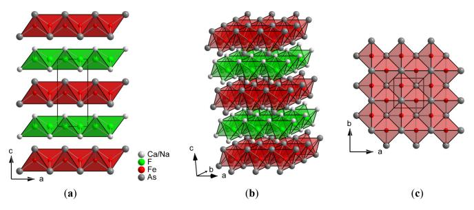
Sodium partly substitutes calcium in  $Ca_{1-x}Na_xFFeAs$  on the 2*c* position. From the four crystallographically independent atoms, iron and fluorine are both tetrahedrally coordinated, whereas arsenic and calcium are surrounded in the form of square antiprisms built from four counter ions of each kind (Figure 3).
