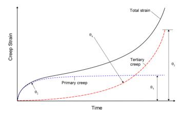
**Figure 2.** Examples of creep curves represented using Equation (1).
