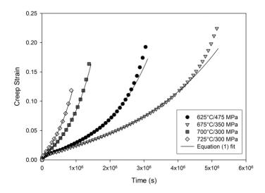
Therefore, when analysing constant stress creep curves, data points after the onset of necking must be ignored and the  $\theta$  coefficients can accordingly be found by minimising the function  $\phi^{n-1}$  of the form:
