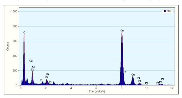
Figure 2. EDX spectrum of the MWCNTs-Pt NPs nanohybrids on copper grids.
