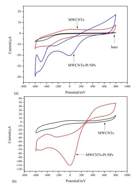
We can detect  $H_2O_2$  at 0 mV as working potential using the MWCNTs/Pt NPs-modified electrode, judging from the CV reported in Figure 3(b). The applied potential for the MWCNTs/Pt NPs-modified electrode is much lower than those for previously-reported  $H_2O_2$  sensors [30–32]. Therefore, the background current may be decreased and the response to interference materials can be minimized.
