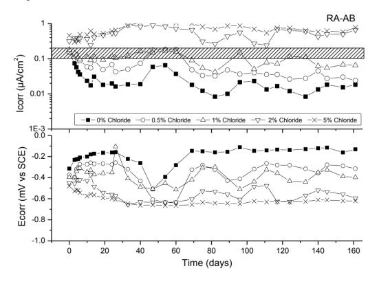
Figure 11 shows corrosion ( $I_{corr}$ ) and corrosion potential ( $E_{corr}$ ) evolution of steel reinforcement embedded in all concrete types when they are exposed to a carbonation attack. This experiment is also divided in three stages similar to sea water attack. The first one is the curing period, to evaluate if steel reinforcement has achieved a passive state, and again, this starting condition was correctly attained.
