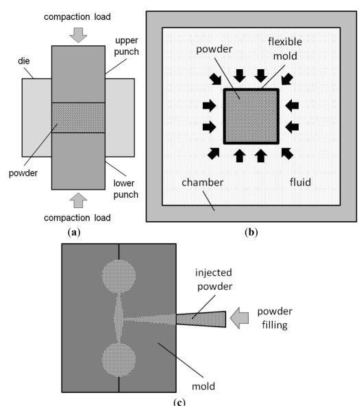
**Figure 9.** Common techniques of compaction in the fabrication of metallic scaffolds with the space holder method: (**a**) uniaxial die pressing; (**b**) isostatic pressing and (**c**) injection molding.
