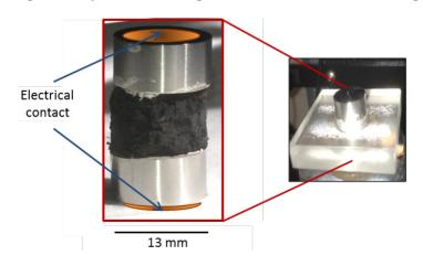
An Instron 5942 with a 100 N load cell (Instron, Norwood, MA, USA), configured to study the material in compression, was employed for all macroscopic tests. The compressive force was selected to remain between 10 and 90 N. The lower limit was selected in order to prevent the carbon nano-fiber from losing contact with the anvil while the upper limit was chosen to prevent reaching the 100 N automatic cutout limit on the load cell used in the test.
