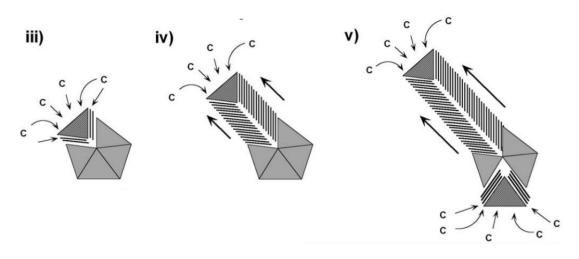
**Figure 4.** Schematic illustration of the typical chemical vapor deposition growth mechanism of the platelet CNFs [15].
