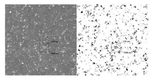
Figure 10. TEM image for the fractal dimension calculation in the carbon/polymer composite [53].
