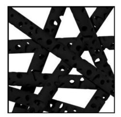
Figure 13. The SEM microstructure of the (a) PPy nanofiber webs and (b) CNF webs [82].
