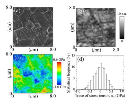
**Figure 5.** Average stress histograms collected on statistically meaningful surface areas of unused biomedical  $Al_2O_3$  materials belonging to two different generations of  $Al_2O_3$  bioceramics for hip joints. The average grain sizes are shown in inset.
