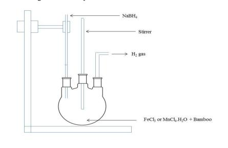
Figure 8. Schematic diagram for the synthesis of nZVI-bamboo and nMn-bamboo composites.
