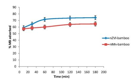
Figure 5. Effect of time (wt = 0.02 g, pH = 5;  $C_0 = 140$  mg/L,  $T = 32 \pm 2$  °C at 165 rpm).
