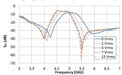
**Figure 5.** LC driving voltage dependence of the  $S_{21}$  parameter for the new bandpass filter.
