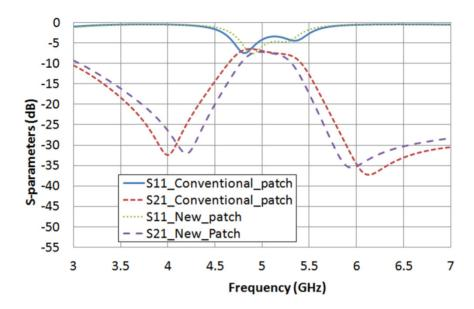
**Figure 11.** S-parameters obtained in simulation for both structures considering  $\varepsilon_{rl} = 3.06$  and  $\tan \delta_l = 0.02$ .
