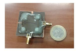
**Figure 4.** Manufactured LC bandpass filter.
