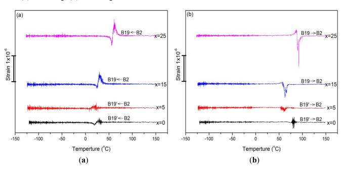
**Figure 5.** The strain variation curves for  $Ti_{50}Ni_{50-x}Cu_x$  SMAs, x = 0, 5, 15, 25 at.% (a) in cooling; (b) in heating.
