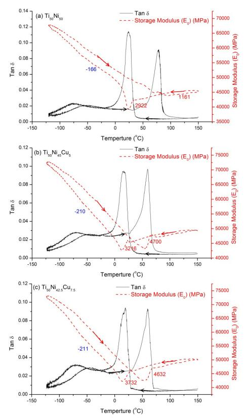
**Figure 2.** The tan  $\delta$  value and storage modulus ( $E_0$ ) curves for Ti<sub>50</sub>Ni<sub>50-x</sub>Cu<sub>x</sub> SMAs. (a) x = 10; (b) x = 12.5; (c) x = 15 at.%. The blue number are the  $E_0$  slopes in B19' and B19 martensites, and the red numbers are the magnitude of  $E_0$  softening and hardening.
