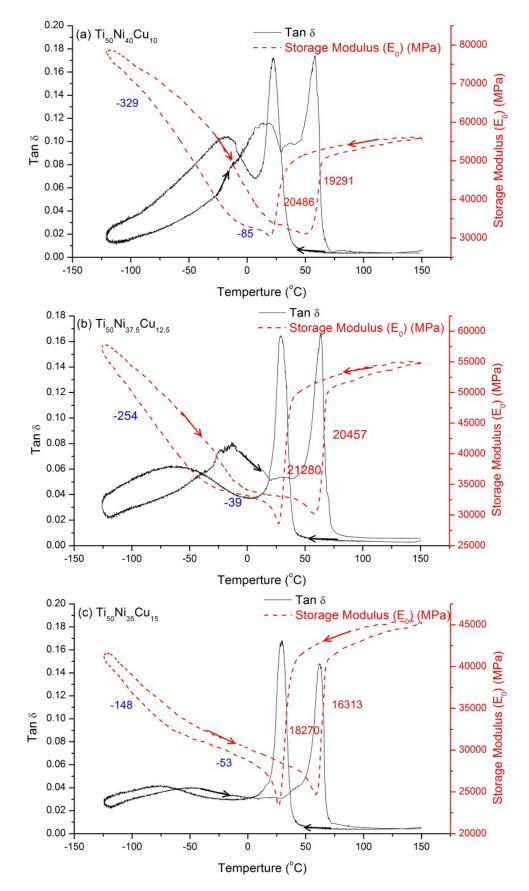
**Figure 3.** The tan  $\delta$  value and storage modulus ( $E_0$ ) curves for Ti<sub>50</sub>Ni<sub>50-x</sub>Cu<sub>x</sub> SMAs. (a) x = 20; (b) x = 25; (c) x = 30 at.%. The blue number is the  $E_0$  slope in B19 martensite, and the red numbers are the magnitude of  $E_0$  softening and hardening.
