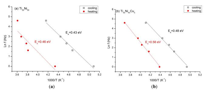
**Figure 6.** The plots of ln frequency *vs.* reciprocal relaxation peak temperature in cooling and heating processes for  $Ti_{50}Ni_{50-x}Cu_x$  SMAs. (a) x = 0; (b) x = 5; (c) x = 7.5 at.%.
