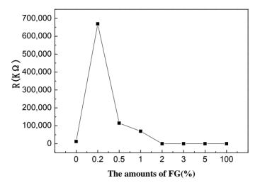
**Figure 10.** Responses of FG/WO<sub>3</sub> nanocomposites sensors with different amounts of FG to 100 ppm  $NO_x$  at different operating voltage.
