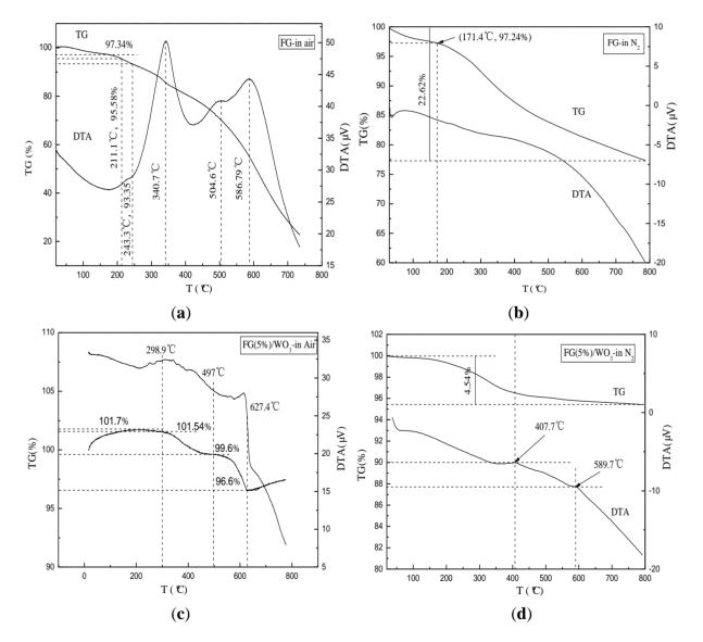
From Figure 7c, it can be seen that the FG  $(5\%)/WO_3$  nanocomposites synthesized via the solvothermal method shows two abrupt weight losses occurring between 300 and 630 °C in air atmosphere. Correspondingly, the DTA curve shows an endothermic peak and an exothermal peak, which can be assigned to the loss of chemically bonded water and oxidation of graphene in air, respectively. As shown in Figure 7d, the TG curve of FG  $(5\%)/WO_3$  nanocomposites performed in
