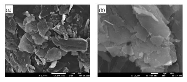
**Figure 2.** Morphology of FG prepared via facile solvothermal route: (**a**) FE-SEM image; and (**b**) TEM image.
