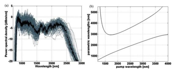
**Figure 7.** (a) Numerically generated evolution of supercontinuum spectrum along the length of PCF; (b) corresponding numerical spectrogram at the output of PCF.
