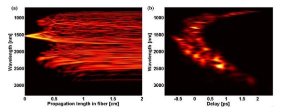
Numerical supercontinuum bandwidth covers a range of 700–2800 nm in a 20 dB range. At about 5 mm of propagation, energy is transferred to sidebands at around 1000 nm and 2400 nm, which quickly merge with the central area. In order to identify these sidebands, we calculated phase-matching condition for the four-wave mixing (FWM) process,  $\kappa = 0$ , where the phase mismatch  $\kappa$  can be expressed as [22]:
