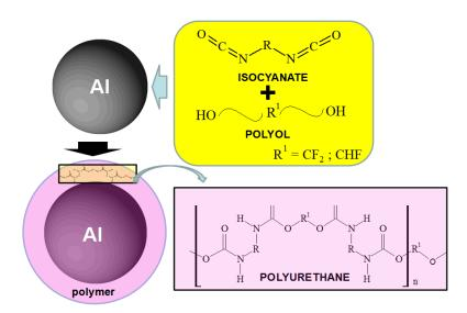
Figure 1. Schematic diagram of the synthesis reaction for the polymer on Al nanoparticles.
