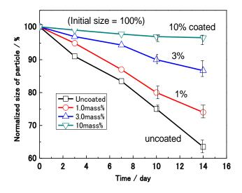
Figure 13. Effect of coating mass% on the hydrogen (H<sub>2</sub>) evolution reaction on Al nanoparticles.
