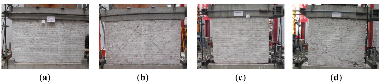
Figure 8. Crack patterns and failure of the specimens: (a) MWA-1; (b) MWB-1; (c) MWA-2; (d) MWB-2; (e) MWA-3; (f) MWB-3; (g) MWA-4; (h) MWB-4.
