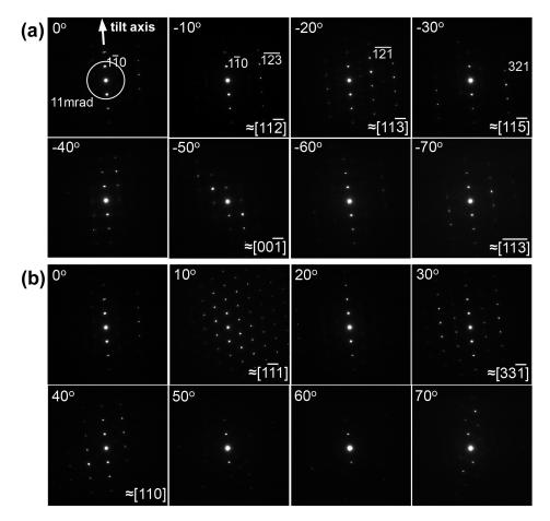
**Figure 1.** Tilt-series of selected area electron diffraction (SAED) patterns obtained from the  $\beta$  phase region in a Ti-35mass%Nb alloy. The *hh*0 systematic reflections are excited parallel to the tilt axis. (a) SAED patterns obtained at tilt angles from 0° to -70°, and (b) those from 0° to 70°.
