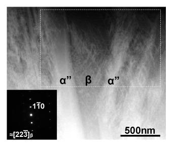
**Figure 4.** Magnified BF-STEM image and corresponding SAED pattern of the Ti–35mass%Nb alloy observed at a stage tilt of 0°. The image contrast is reversed in order to clearly show fine dislocations. The beam incidence is close to the  $[22\overline{3}]_{\beta}$ . The rectangular area indicated by dashed lines was selected for subsequent 3D reconstruction.
