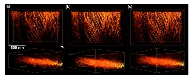
**Figure 7.** Effects of low contrast images and the maximum tilt angles on shapes and width of reconstructed dislocations. The maximum tilt angles and the number of images used for the reconstruction are as follows: (**a**) 70°, 63 images, (**b**) 70°, 71 images, (**c**) 40°, 41 images. An arrow indicates the viewing direction of the attached cross section images.
