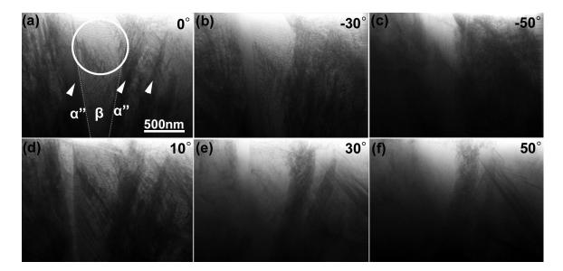
**Figure 3.** Snapshots of bright-field scanning transmission electron microscopy (BF-STEM) images of the as-quenched Ti–35mass%Nb alloy acquired during a tilt-series observation. SAED patterns were observed from a circular area indicated in (**a**). Arrowheads indicate acicular  $\alpha$ " martensite plates. Dotted lines indicate  $\alpha$ "/ $\beta$  grain boundaries. Tilt angles for each image is as follows: (**a**) 0°, (**b**) –30°, (**c**) –50°, (**d**) 10°, (**e**) 30°, (**f**) 50°.
