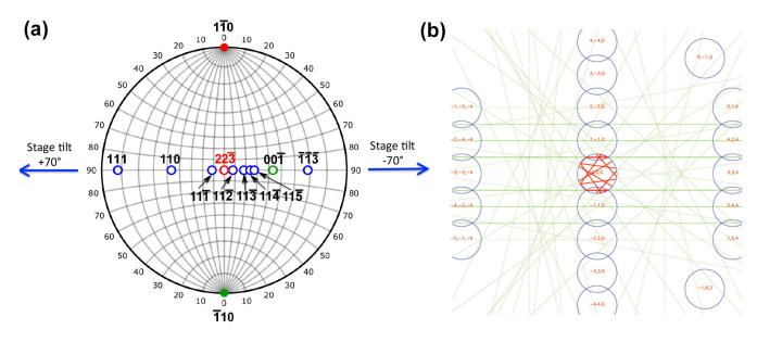
**Figure 2.** (a) Stereographic projection indicating changes of zone axes as a function of stage tilt angle. The initial beam incidence is close to  $[223]_{\beta}$ , and both 110 and 110 reflections are always excited during the tilt series acquisition; (b) A simulated convergent-beam electron diffraction (CBED) pattern with the  $[223]_{\beta}$  zone.
