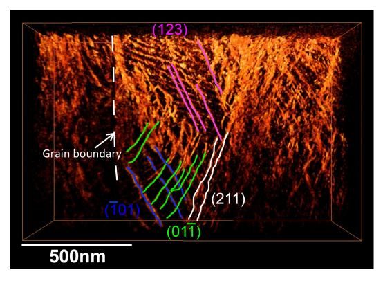
**Figure 6.** A result of slip plane analyses: dislocations on different slip planes are marked by different colors.
