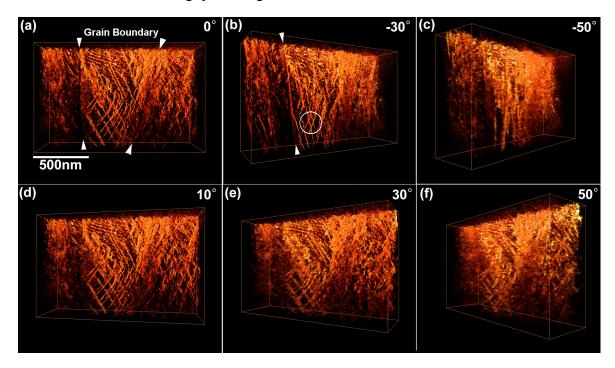
**Figure 5.** Three-dimensional views of the dislocations reconstructed from a BF-STEM tilt-series dataset using a weighted back-projection (WBP) technique. Arrowheads indicate the  $\alpha''/\beta$  grain boundary. A kink on a (101) slip plane is seen in the encircled area. Tilt angles for each image is as follows: (a) 0°, (b) -30°, (c) -50°, (d) 10°, (e) 30°, (f) 50°.
