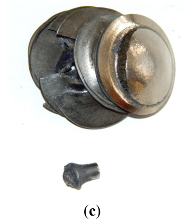
Figure 27. (a) A scheme of metallic/intermetallic laminate composed of aluminum alloy and Ti–Al intermetallic alloy (based on [151]), and (b) a SEM microphotograph of \text{Ni}_3\text{Al} multilayer material (eight \text{Ni}_3\text{Al} plates obtained by explosive welding) [136]; (c) a pack of a \text{Ni}_3\text{Al} (Zr, B) plates (packed loosely) after a shooting test with 7.63 mm caliber bullet (kbbk AK 47) with a view of deformed bullet core [118].
