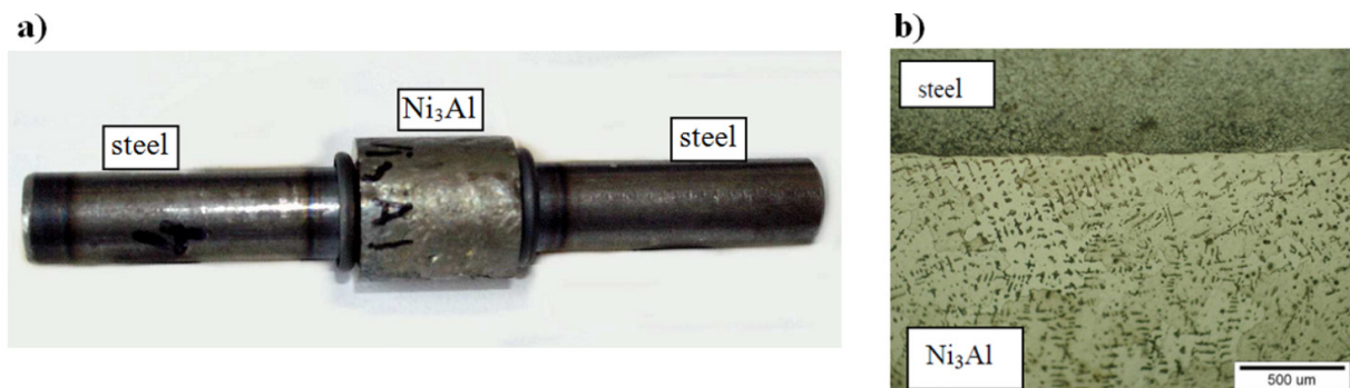
Figure 5. The \text{Ni}_3\text{Al} /steel joints obtained by a friction welding technique. (a) A macroscopic view and (b) a microstructure image [65].
