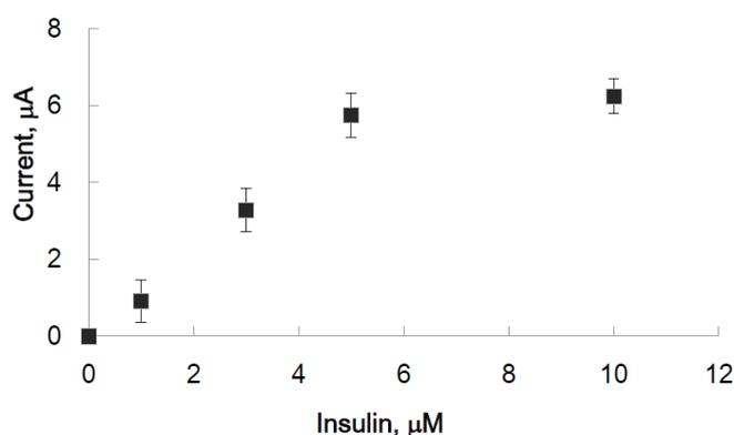
**Figure 6.** Calibration plot of current difference to insulin concentration. The cathodic peak current difference between the state with and without insulin was plotted *versus* insulin concentration. The concentration of  $\text{H}_2\text{O}_2$  was 20  $\mu\text{M}$ .
