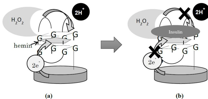
**Figure 1.** Scheme of insulin sensing utilizing a G-quadruplex immobilized electrode: (a) measurement of peroxidase activity with the aid of hemin without insulin; (b) measurement of peroxidase activity after binding to insulin.
