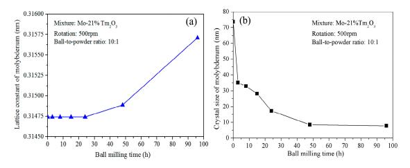
**Figure 2.** (**a**) Curve of the lattice parameter of Mo vs. ball-milling time; and (**b**) curve of the crystalline size of Mo vs. ball-milling time.
