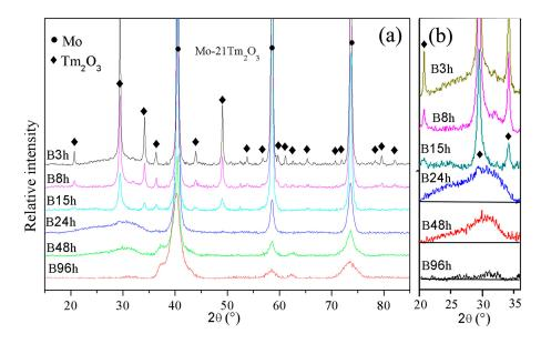
**Figure 1.** (a,b) X-ray patterns of Mo (21 wt %)  $Tm_2O_3$  powder mixtures milled for different times at a 20 of  $15^{\circ}$ – $85^{\circ}$  and  $20^{\circ}$ – $36^{\circ}$ , respectively.
