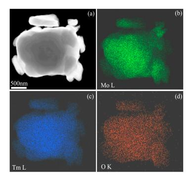
**Figure 4.** STEM analysis results of Mo (21 wt %) Tm<sub>2</sub>O<sub>3</sub> powder mixtures milled for 96 h; (**a**) high angle annual dark field STEM image; (**b**–**d**) Mo L, Tm L, and O K element mappings, respectively.
