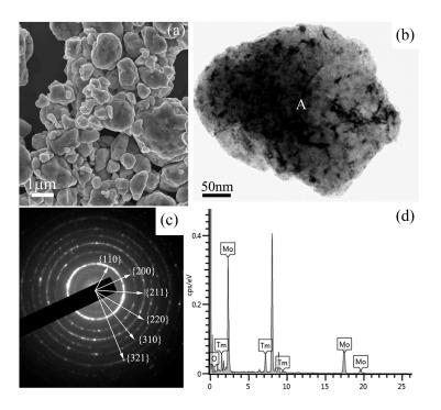
**Figure 3.** Microstructure analysis results of Mo (21 wt %)  $Tm_2O_3$  powder mixtures milled for 48 h; (a) SEM image showing the morphology of the ball-milled powders; (b) bright field TEM image; (c) selected area electron diffraction pattern from region 'A' in (a) showing the Mo phase; and (d) EDS analysis results from region 'A' in (a) showing the diffraction peaks of Tm, Mo, O, and Cu elements. Cu peaks comes from the copper grid.
