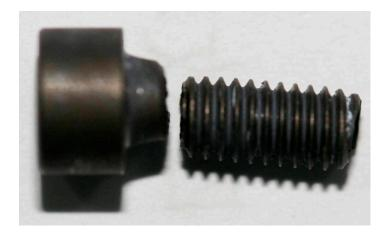
Figure 1. Fracture position of screw.
