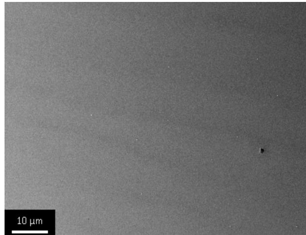
**Figure 5.** Low-resolution electron micrograph of TiO<sub>2</sub> gel layer deposited after one dip-coating cycle.
