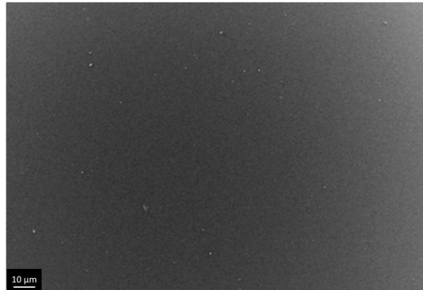
**Figure 9.** Microphotographs of  $\text{TiO}_2$  film with a thickness of 33 nm after shock drying, obtained at low resolution.
