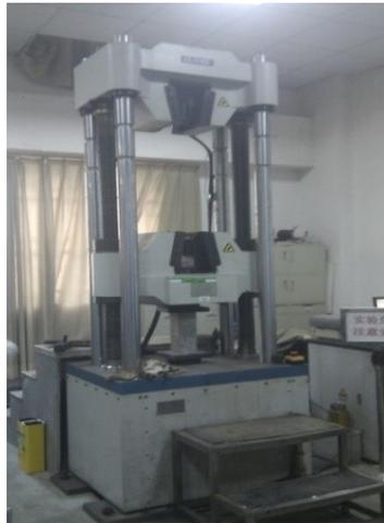
Figure 3. Hydraulic servo testing machine.
