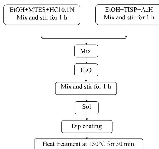
**Figure 7.** Flow chart of the preparation process of SiO<sub>2</sub>-TiO<sub>2</sub> thin films.
