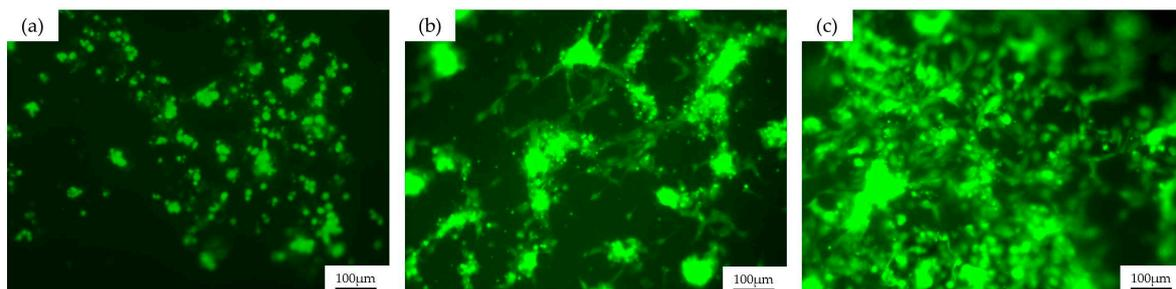
**Figure 6.** Representative fluorescence microscopy images of the different sol-gel-coated channels with HUVECs stained with calcein AM after a one-day culture. (a) PDMS channel with 60MTES/40TEOS coating; (b) with 70MTES/30TISP coating; and (c) with 80MTES/20TISP sol-gel coating.
