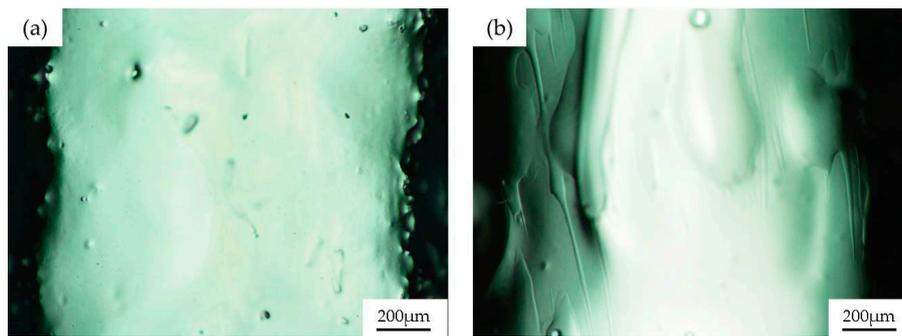
**Figure 5.** Microscopy images of PDMS channel: (a) uncoated and (b) with sol-gel coating.
