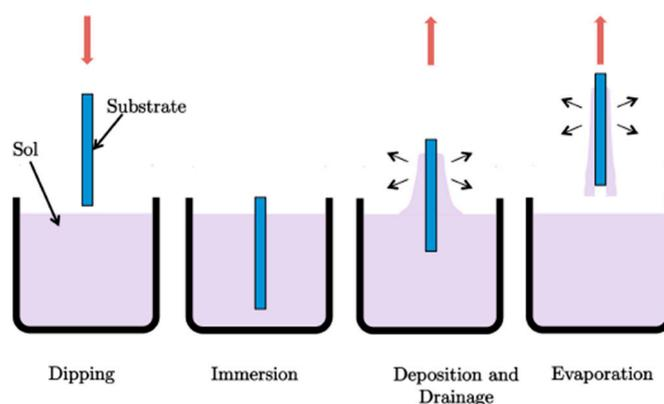
**Figure 4.** Deposition by the dip-coating technique: dipping and immersion of the substrate into the sol, formation of the layer by withdrawing the substrate and gelation of the layer by solvent evaporation.
