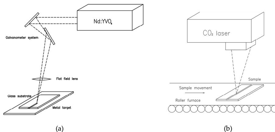
**Figure 1.** Experimental setups employed for the fabrication of the channel over soda-lime glass. Schemes of (a) the fabrication of the channel; and (b) the subsequent thermal treatment to reduce the roughness of the structure.
