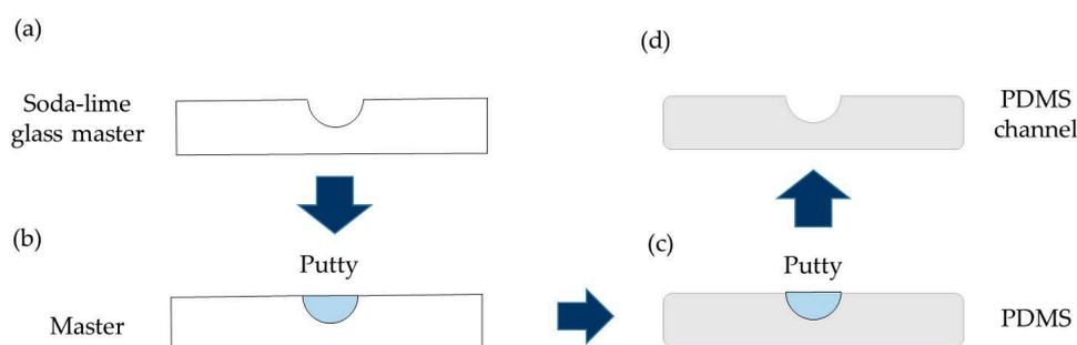
**Figure 2.** Scheme of the replication process. (a) Soda-lime glass master fabricated by laser techniques; (b) The putty is placed inside the channel to obtain the inverse structure of the master; (c) The putty mold is covered with PDMS and cured; (d) Finally, after peeling off the PDMS, the final channel is obtained.
