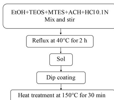
**Figure 8.** Flow chart of the preparation process  $\text{SiO}_2$  layers using MTES and TEOS.
