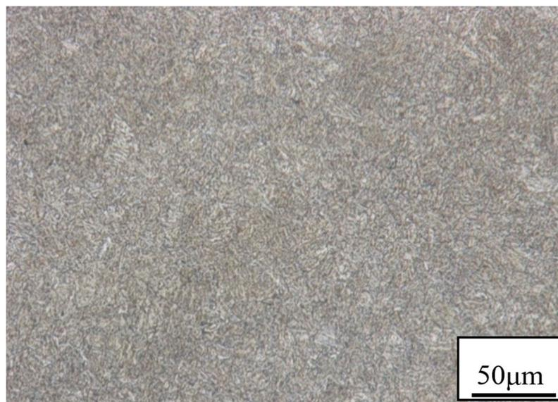
Figure 1. Microstructure of L80 steel.
