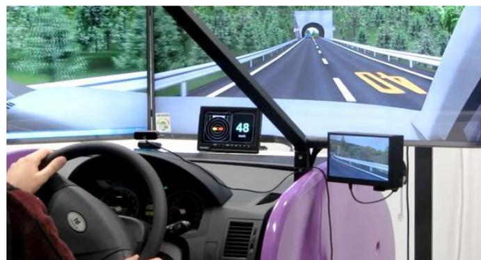
**Figure 2.** Experimental environment: full-scale Forum-8 drive simulator.
