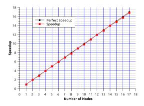
**Figure 5.** Speed-up obtained in the cluster. The perfect speedup is 17 and the obtained speedup is 16.85, giving us a very good performance.
