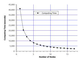
**Figure 4.** Computing times obtained from 1 to 17 processes in the cluster; the processes follow an ordered affinity.
