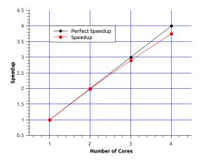
**Figure 3.** Speed-up obtained in one node. As can be observed the speed-up is almost linear. The computing times are 154,158 s, 77,395 s, 53,214 s and 41,082 s.
