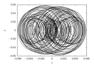
(a) Chaotic trajectory with initial conditions given by  $(x, \theta, \phi, \dot{x}, \dot{\theta}, \dot{\phi}) = (-0.007, -1.3439, \pi/2, 0, 0, 0).$
