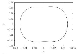
(**b**) Non-chaotic trajectory with initial conditions given by  $(x, \theta, \phi, \dot{x}, \dot{\theta}, \dot{\phi}) = (0, \pi/2, \pi/2, 0, 0, 0).$
