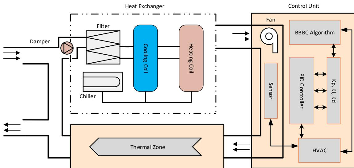
Figure 3. Block diagram of conventional HVAC system and control unit structure.
