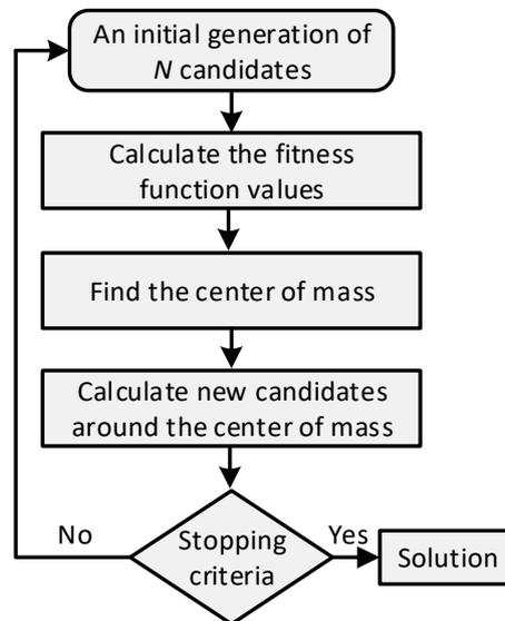
Figure 2. BB–BC optimization algorithm flow chart.
