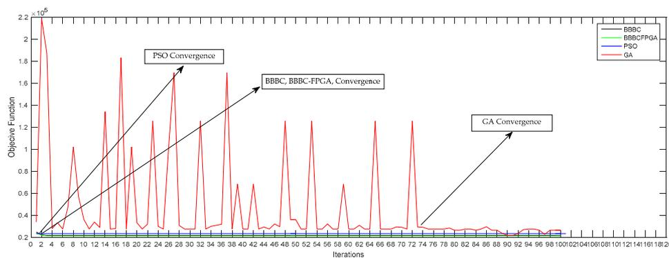
**Figure 13.** Objective function convergence for all four optimization methods.
