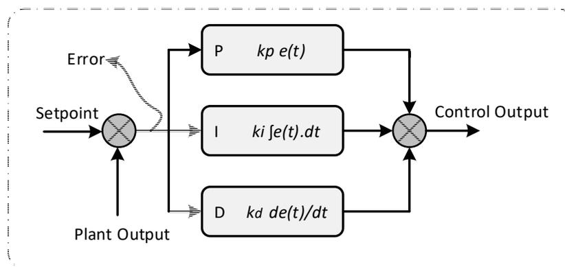
Figure 1. Block diagram of typical PID control structure.
