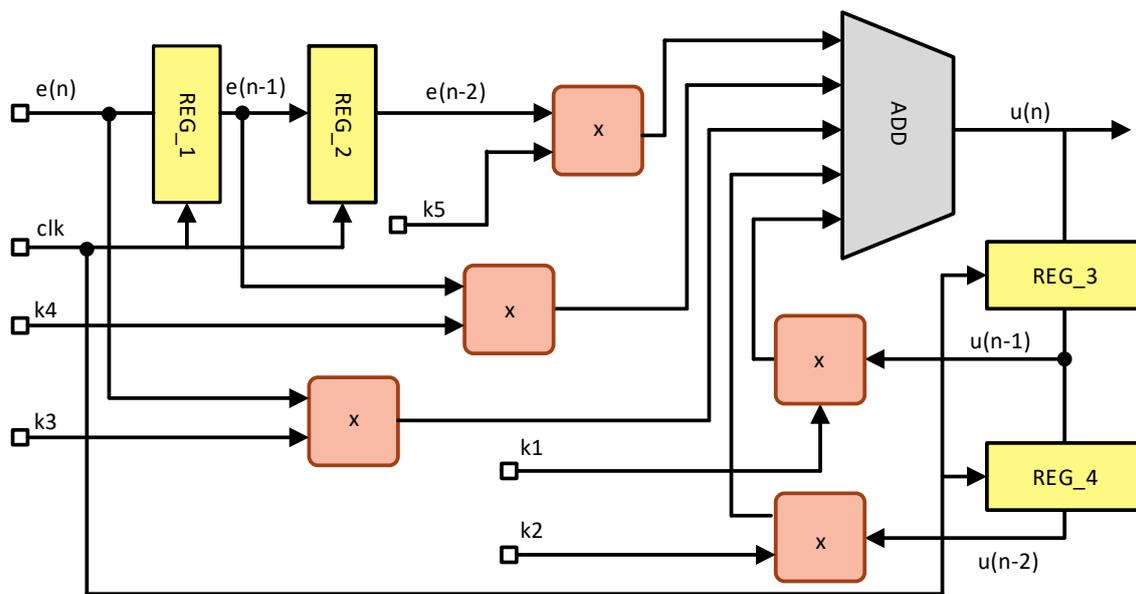
Figure 5. Block diagram of a typical PID controller FPGA architecture.
