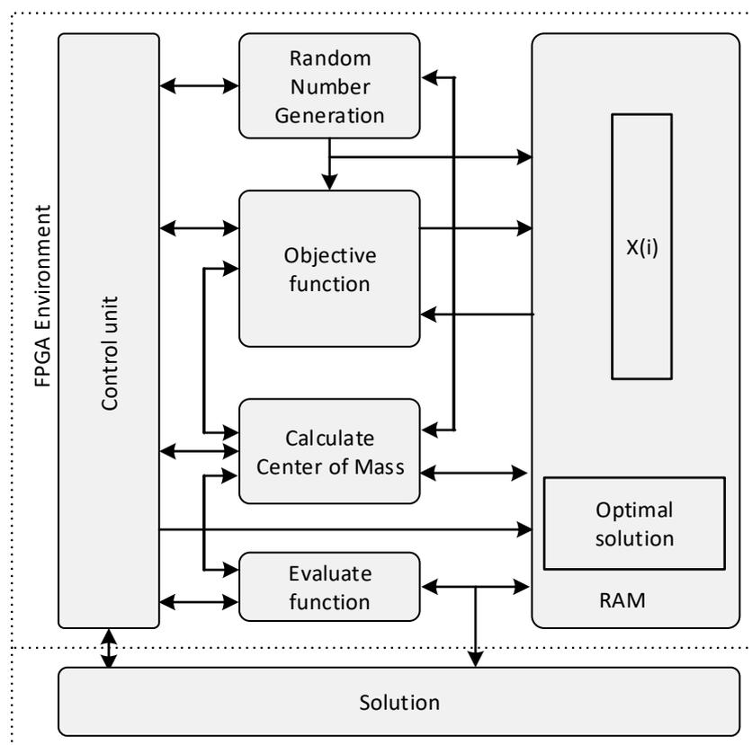
Figure 6. Top-level diagram of the BB-BC FPGA architecture.
