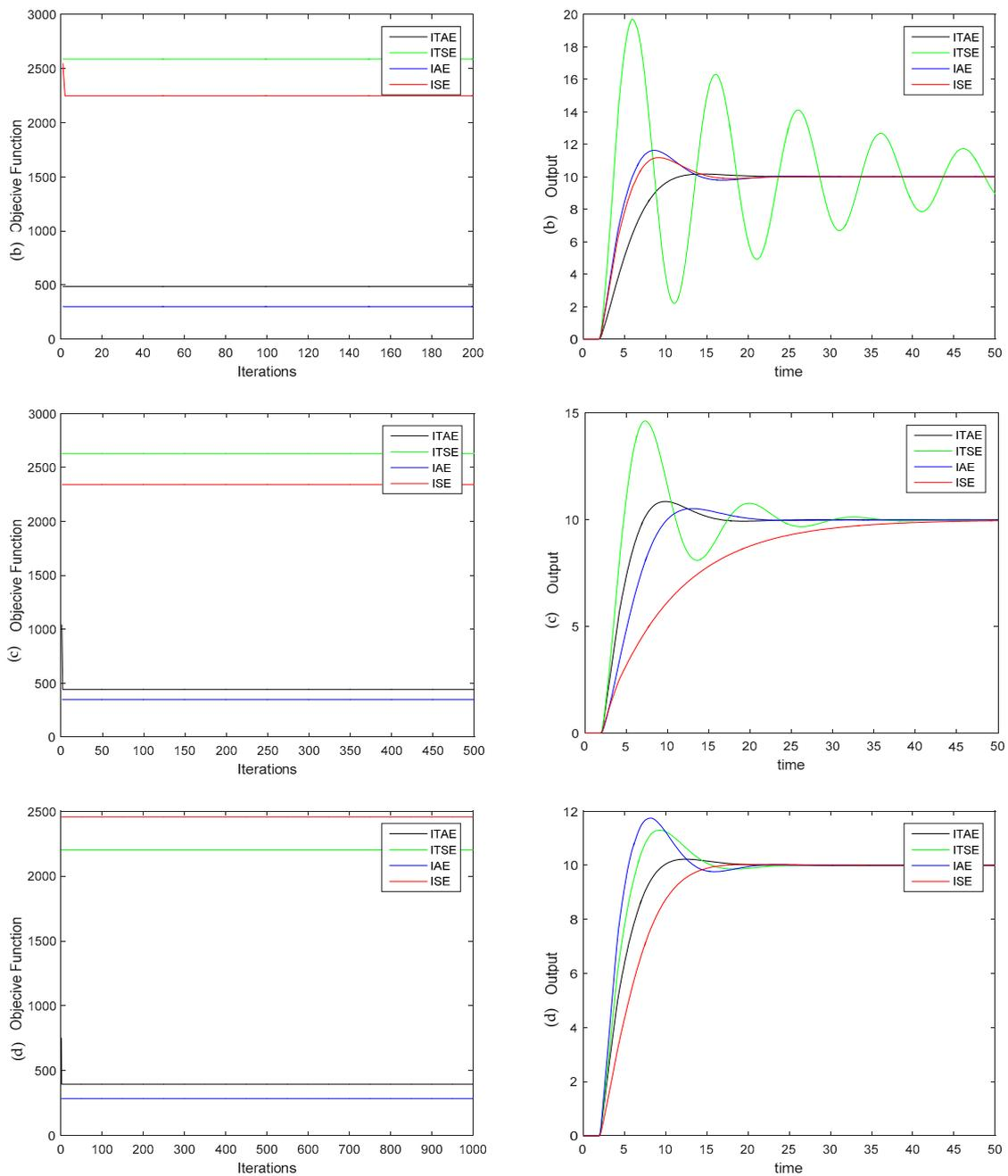
**Figure 4.** Convergence and time response of the widely used objective function in controller tuning via optimization (*ITAE*, *ITSE*, *IAE*, *ISE*) for different number of iterations (a) 100, (b) 200, (c) 500 and (d) 1000 iterations.
