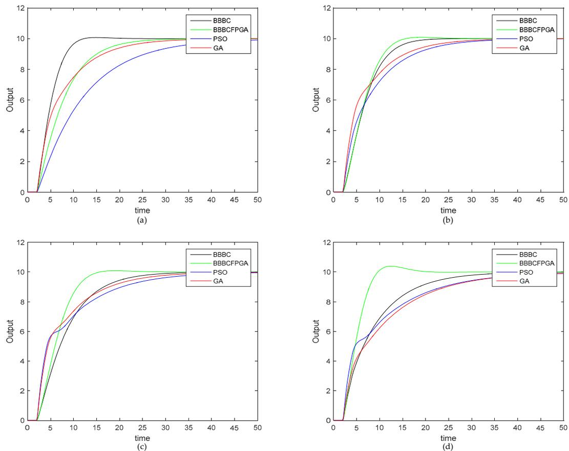
**Figure 10.** Time responses of four optimization methods (BBBC, BBBC-FPGA, PSO, GA) for different number of iterations (a, b, c, and d for 100, 200, 500, and 1000 iterations, respectively).
