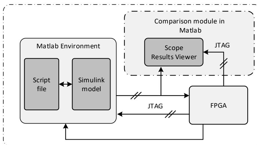
**Figure 7.** FPGA-in-the-loop (FIL) acceleration scheme.
