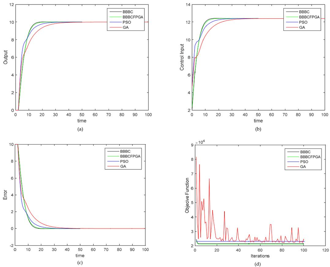
**Figure 11.** The (a) system output, (b) control signal, (c) error signal, and (d) objective function for all four optimization methods.
