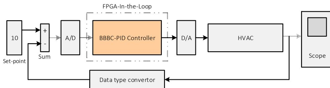
Figure 9. Block diagram of our MATLAB/Simulink model.
