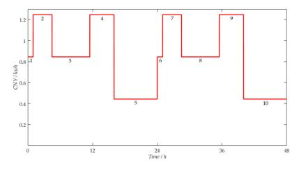
Figure 2. An illustration of the first type of time-of-use (TOU) electricity tariffs.
