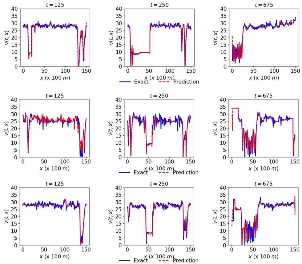
**Figure 7.** Actual and predicted speed at three different times 125, 250, and 675 respectively given by the first, second, and third columns. The first, second, and third rows respectively represent the network’s links L1, L2, and L3.
