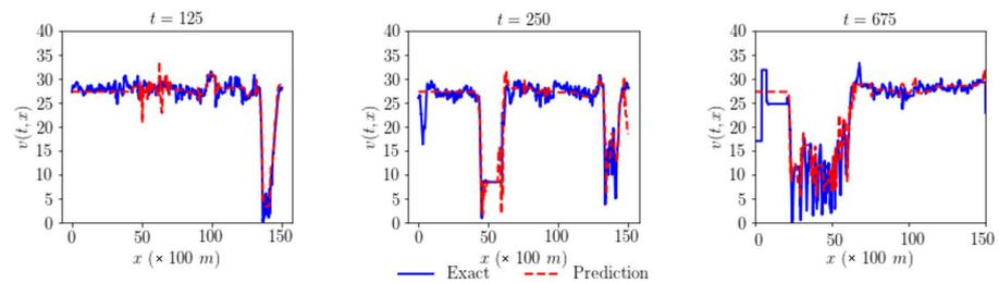
Figure 10. Actual and predicted speed at three different time intervals of Link L3 with adaptive activation function.
