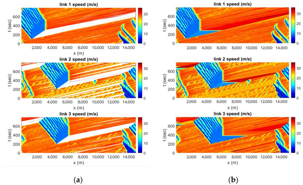
**Figure 4.** (a) Speed contour plot showing cells where no vehicle detected; (b) speed contour where missing cells filled with the speed of neighboring cells.
