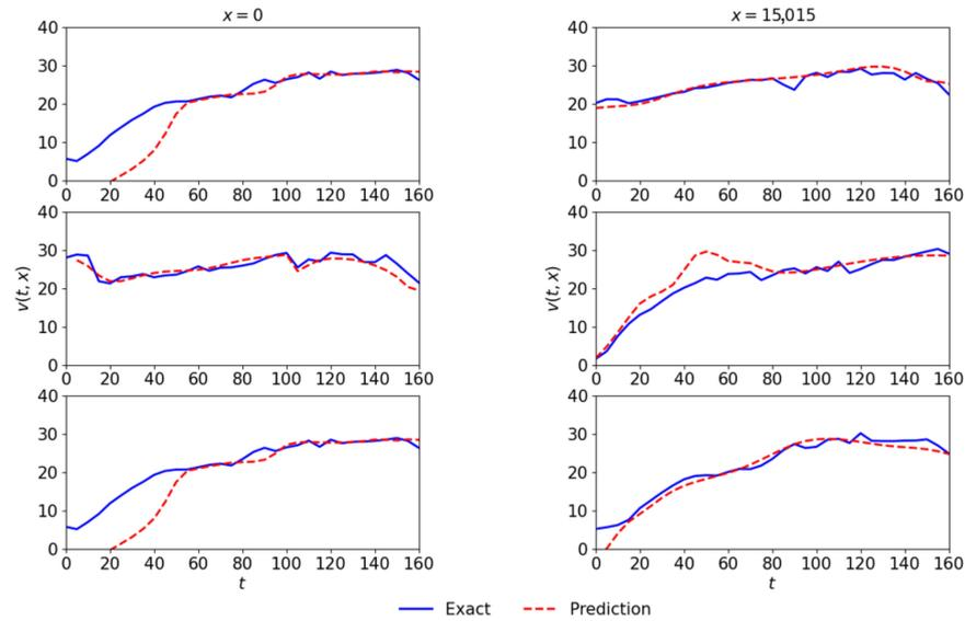
**Figure 12.** Actual and predicted speed at two intersections i.e., at  $x = 0$  and  $x = 15,015$  m, respectively given by the first and second columns. The first, second, and third rows respectively represent the network’s links L1, L2, and L3.
