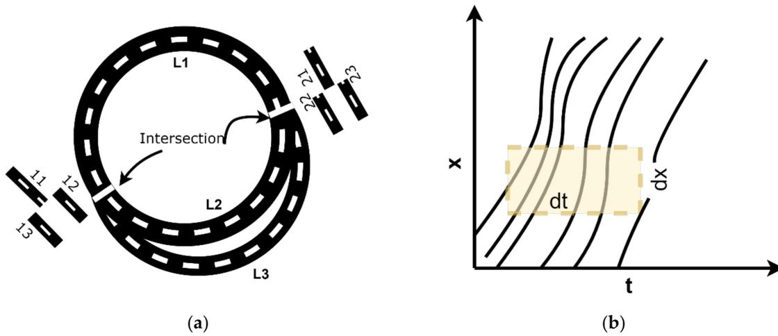
**Figure 3.** (a) Traffic network with three links and two intersection points; (b) the trajectories of the vehicles and a discrete area to estimate the traffic states.
