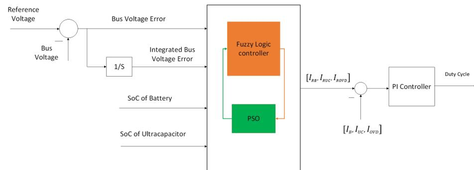
**Figure 5.** Configuration of fuzzy controller, where  $I_B$  is battery current,  $I_{UC}$  is supercapacitor current,  $I_{OVD}$  is OVD current,  $I_{RB}$  is battery reference current, and  $I_{RUC}$  is supercapacitor reference current.
