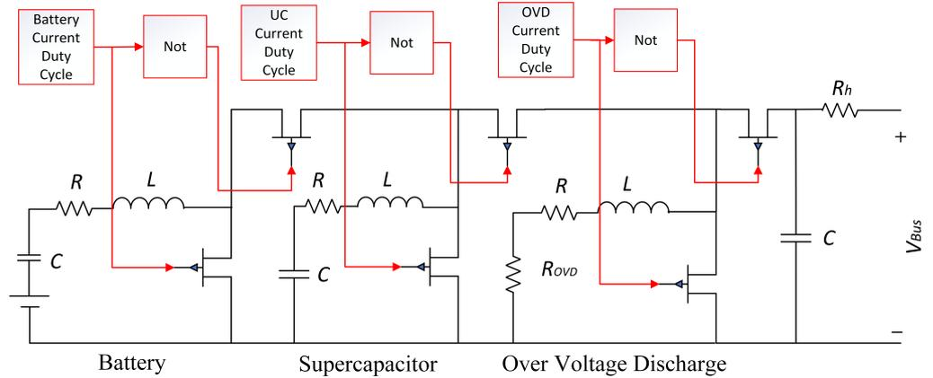
**Figure 4.** Stabilizer model, where  $R$  is the buck–boost converter resistor,  $L$  is the buck–boost converter inductance,  $C$  is the DC link capacitor,  $R_h$  is the connection resistor, and  $V_{Bus}$  is the DC microgrid bus voltage [35].
