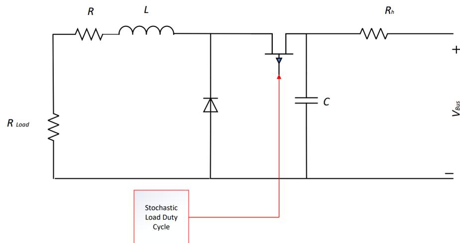
**Figure 3.** Load model, where  $R_{Load}$  is the stochastic load model,  $R$  is the buck converter resistor,  $L$  is the buck converter inductance,  $C$  is the DC link capacitor,  $R_h$  is the connection resistor, and  $V_{Bus}$  is the DC microgrid bus voltage [35].
