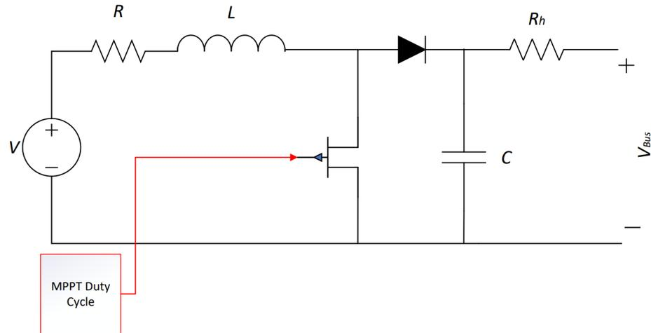
**Figure 2.** Power source model, where  $R$  is the boost converter resistor,  $L$  is the boost converter inductance,  $C$  is the DC link capacitor,  $R_h$  is the connection resistor, and  $V_{Bus}$  is the DC microgrid bus voltage [35].
