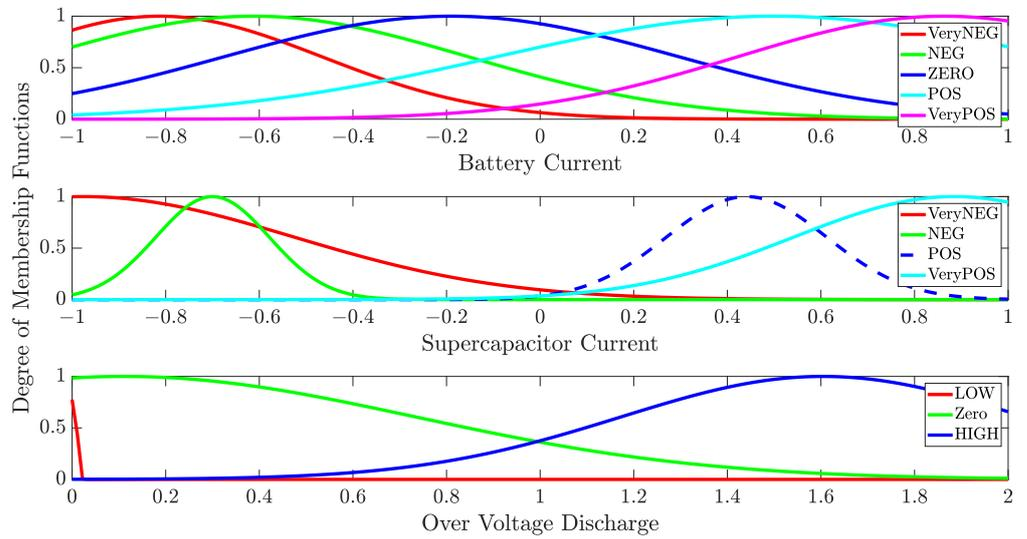
Figure 10. Membership functions for the EV's battery, ultracapacitor, and OVD after optimization.
