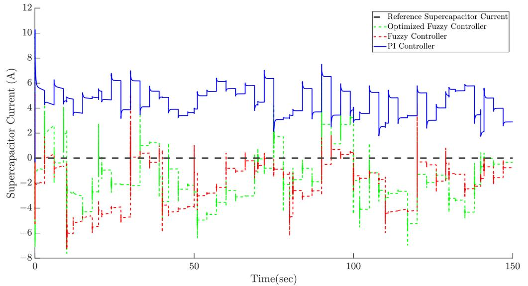
**Figure 15.** The current of the ultracapacitor in three scenarios.
