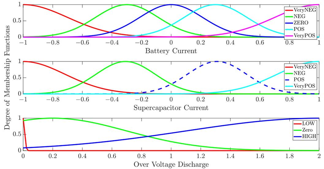
**Figure 8.** Membership functions for the EV’s battery, ultracapacitor, and OVD.
