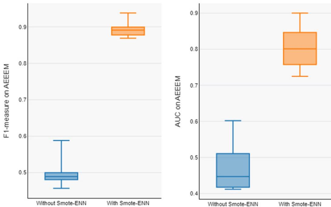
**Figure 5.** Boxplot of F1-measure and *AUC* of model with and without Smote-Enn on AEEEM.
