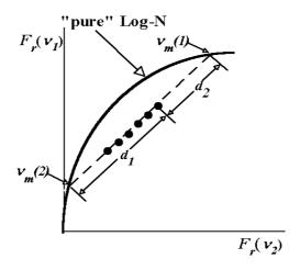
The main limitation of the PHREQ algorithm is that it can only decompose a spectrum into two components. If the correct solution has indeed two-components, the results of the PHREQ analysis correlate with high accuracy to the results obtained by the SIMS algorithm.
