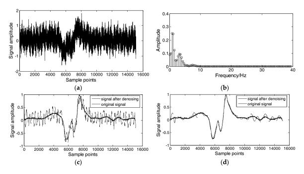
**Figure 8.** Comparison of two noise reduction methods for joint electromagnetic signal: (a) Joint electromagnetic signal with noise; (b) Normalized spectrum diagram of joint signal; (c) Denoised result by improved threshold wavelet; (d) Denoised result by combined use of improved threshold wavelet and EMD.
