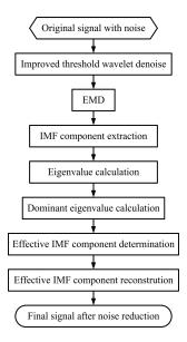
Figure 5. Noise reduction flow chart of combined method of improved wavelet and EMD.
