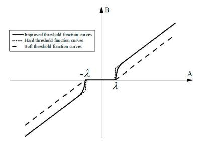
Figure 3. Three kinds of threshold function curve.
