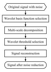
Figure 2. Wavelet threshold noise reduction flow chart.
