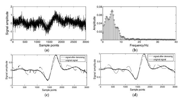
**Figure 9.** Comparison of two noise reduction methods for wire rope break electromagnetic signal: (a) Electromagnetic signal with noise of wire rope break; (b) Normalized spectrum diagram of wire rope break; (c) Denoised result by the improved threshold wavelet; (d) Denoised result by combined use of improved wavelet and EMD.
