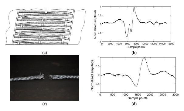
**Figure 7.** Joint and break of steel cord conveyor belt and responding electromagnetic signal: (a) Internal structure of conveyor belt joint; (b) Electromagnetic signal at joint; (c) Steel wire rope break of belt; (d) Electromagnetic signal of wire rope break defect.
