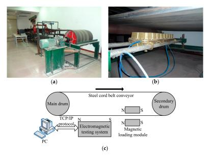
**Figure 6.** Electromagnetic testing rig of steel cord conveyor belt: (a) Tested belt conveyor prototype; (b) Installed electromagnetic testing device; (c) Electromagnetic testing system setup.
