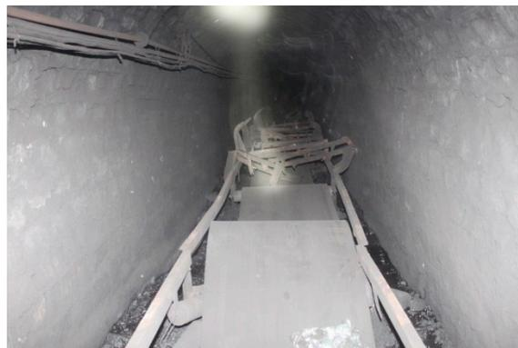
**Figure 1.** Steel cord conveyor belt break scene.
