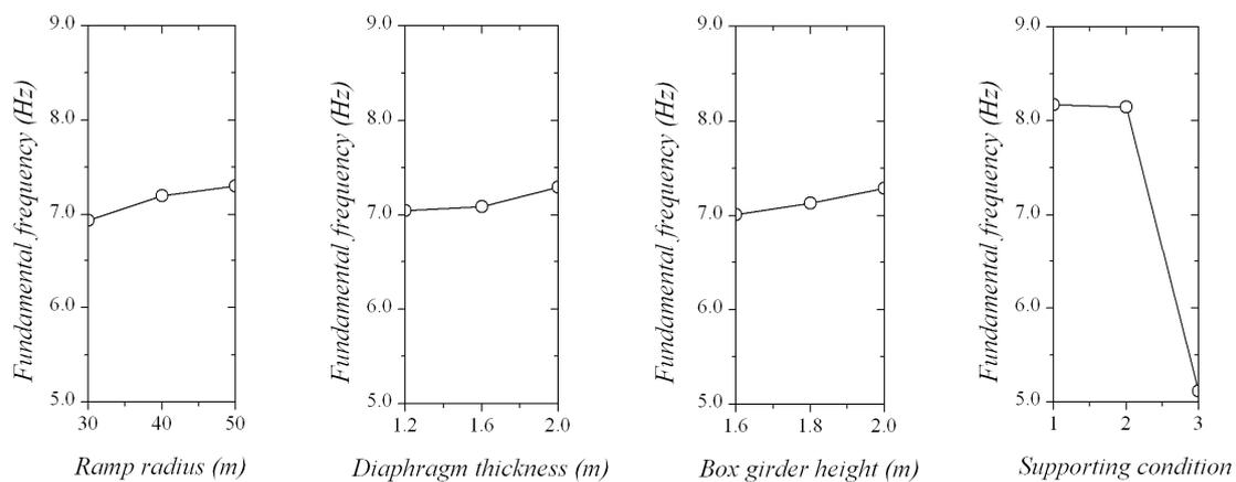
**Figure 9.** Influence of varying parameters on the torsion vibration fundamental frequency.
