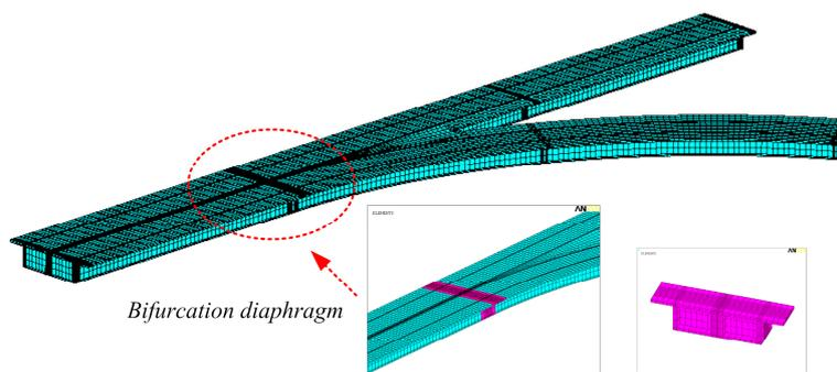
Figure 5. Finite element model of a typical irregularly-shaped bridge.
