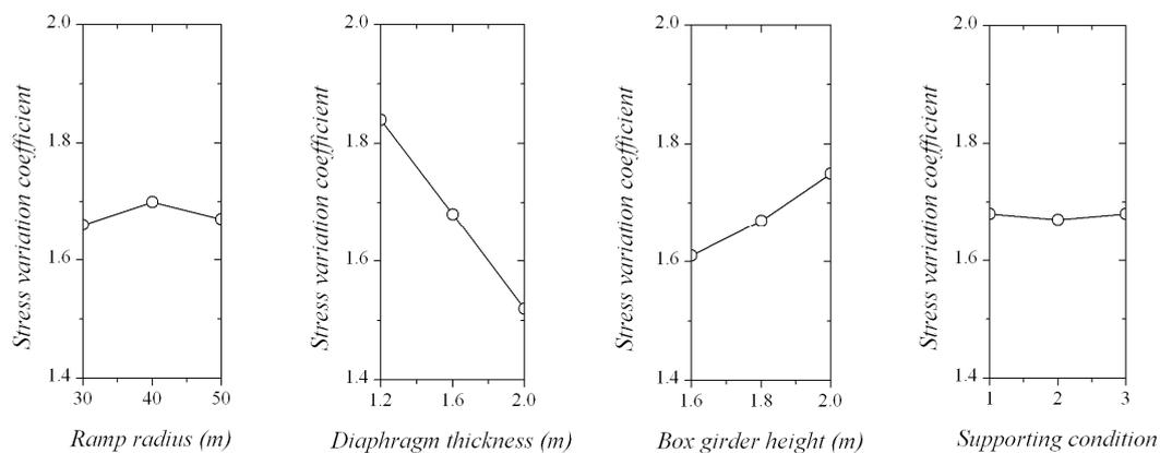
Figure 8. Influence of varying parameters on the stress variation coefficient.
