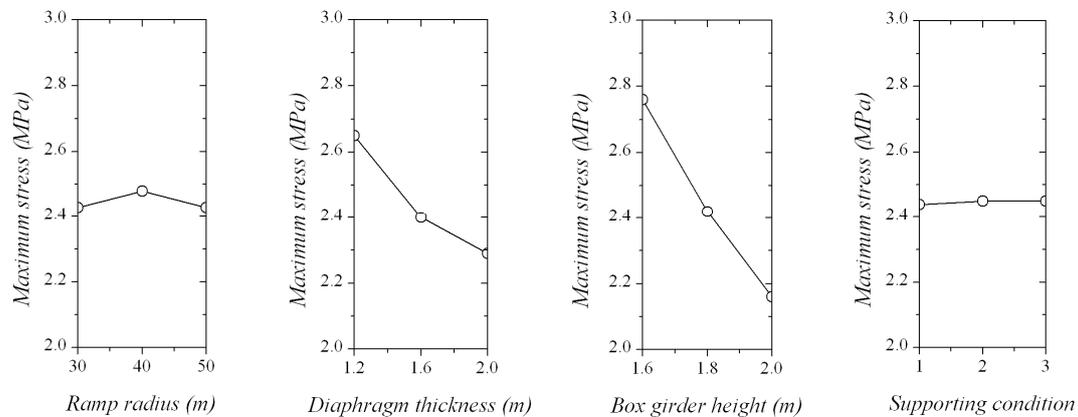
Figure 7. Influence of varying parameters on maximum stress.
