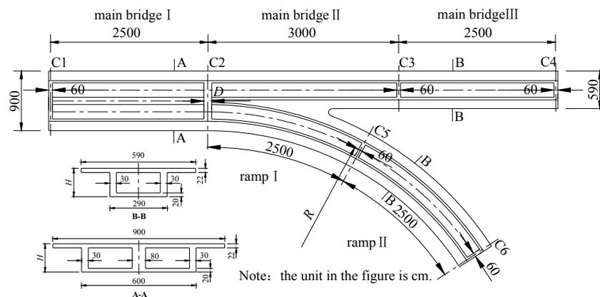
Figure 4. Plan view of a typical irregularly-shaped bridge.
