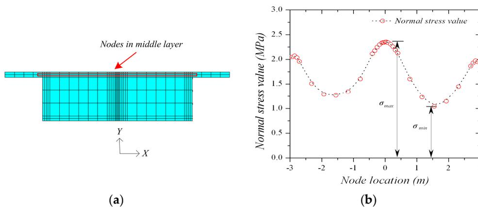
**Figure 6.** Node selection and normal stress distribution in the top plate of the bifurcation diaphragm. (a) Node selected in the top plate; and (b) the normal stress distribution of selected nodes.
