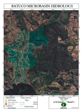
**Figure 2.** Water supply system (light blue), water intake area (red dot), and supply pumps (yellow square) of Batuco Water Committee, Global Positioning System (GPS) points (yellow triangle). Source: Compiled by authors from www.bosquesyagua.cl and field study.
