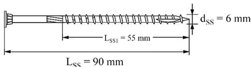
Figure 1. Self-tapping screw specifications.
