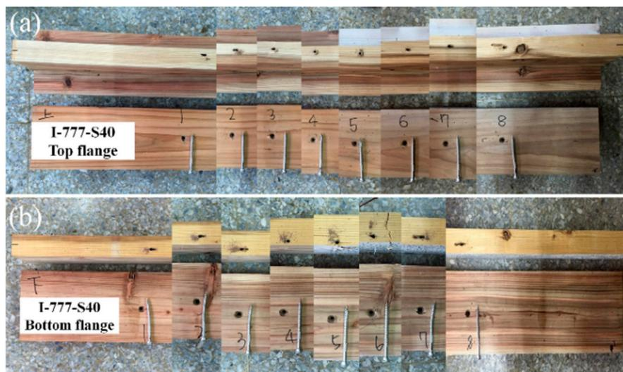
**Figure 10.** Distortional deformation of the screws of the built-up I-beam (a) the top flange of I-777-S40; (b) the bottom flange of I-777-S40.
