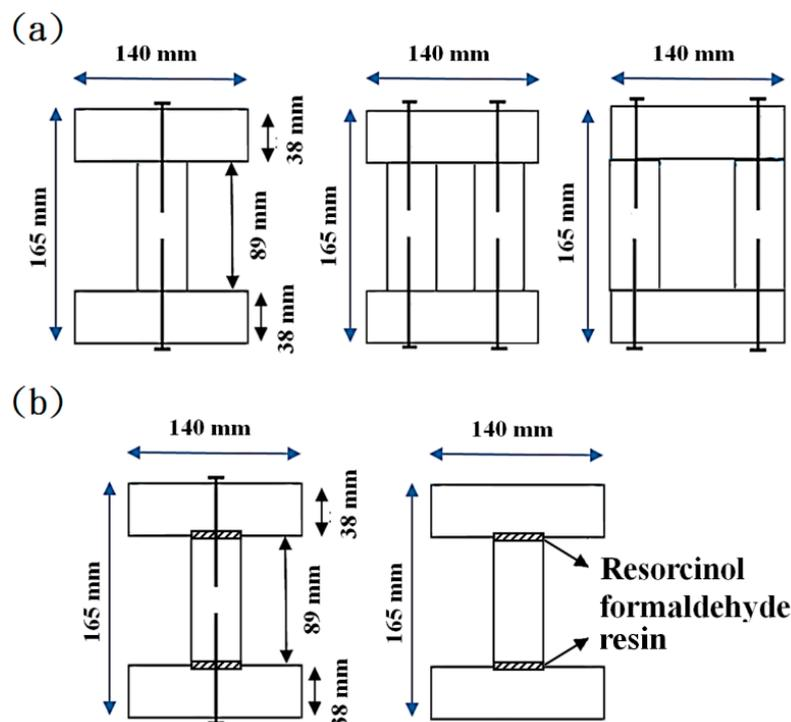
Figure 2. Cross-sectional shapes of built-up beams using (a) self-tapping screws and (b) glue and screws.
