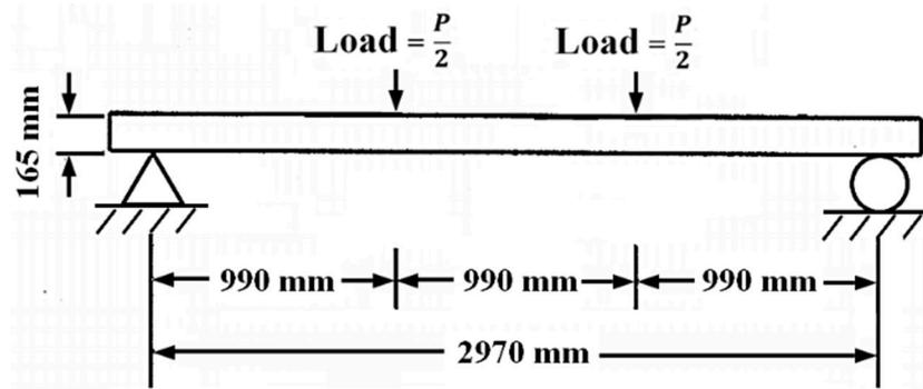
Figure 4. The 4-point bending test scheme.
