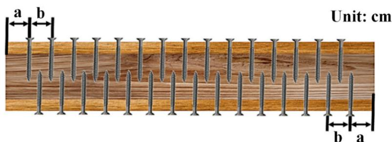
Figure 3. Self-tapping screw drive-in positions.
