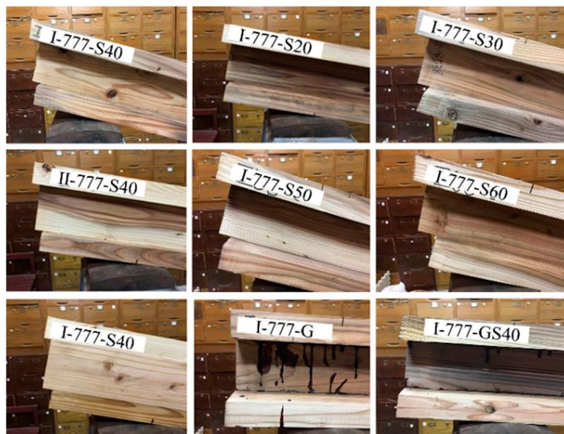
**Figure 9.** End slip of the built-up beams.
