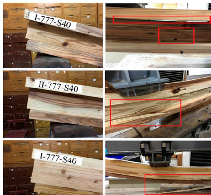
**Figure 6.** Failure usually resulting from the bottom flange at the position directly below the loading position.
