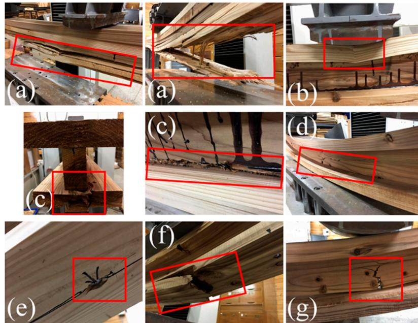
**Figure 7.** Failure modes of the developed built-up and glulam beams: (a) tensile failure at bottom of glulam, (b) compression failure at top flange, (c) failure at wood on glued surface, (d) horizontal shear failure at the web, (e) crushing on the surface using self-tapping screws, (f) failure at knot, and (g) crack at the self-tapping screw joint location.
