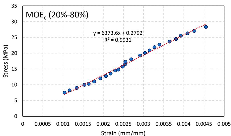
**Figure 9.** Determination of  $MOE_c$  in the 20%–80% interval (specimen A1).
