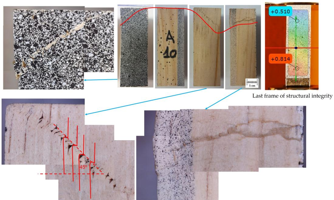
**Figure 20.** Appearance of the damage produced in the specimen A10. Comparison with the last frame of the structural integrity of the sample.
