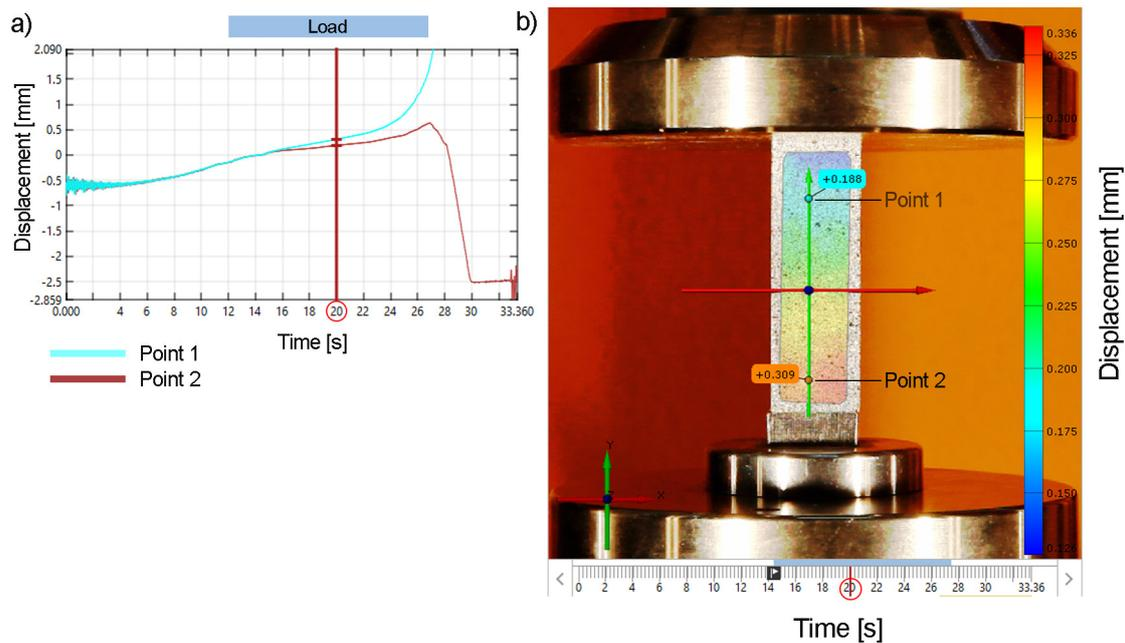
**Figure 6.** (a) Displacement/time diagram of points 1 and 2 and (b) displacement color map of test piece A1.
