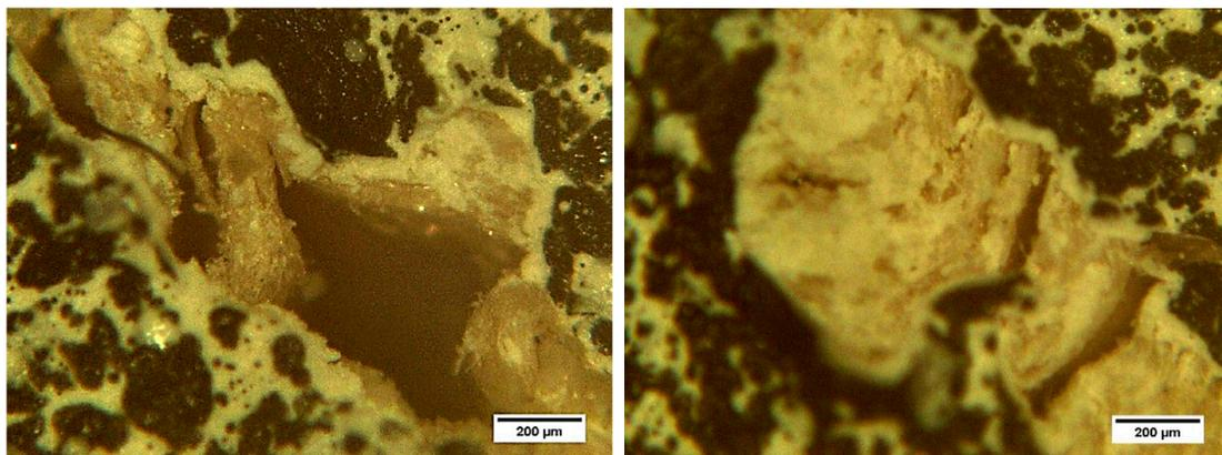
**Figure 18.** Micrographs of the breaking zone of specimen A3 by the speckled zone that was generated at 45°; the consecutive jumps of the fibers are observed.
