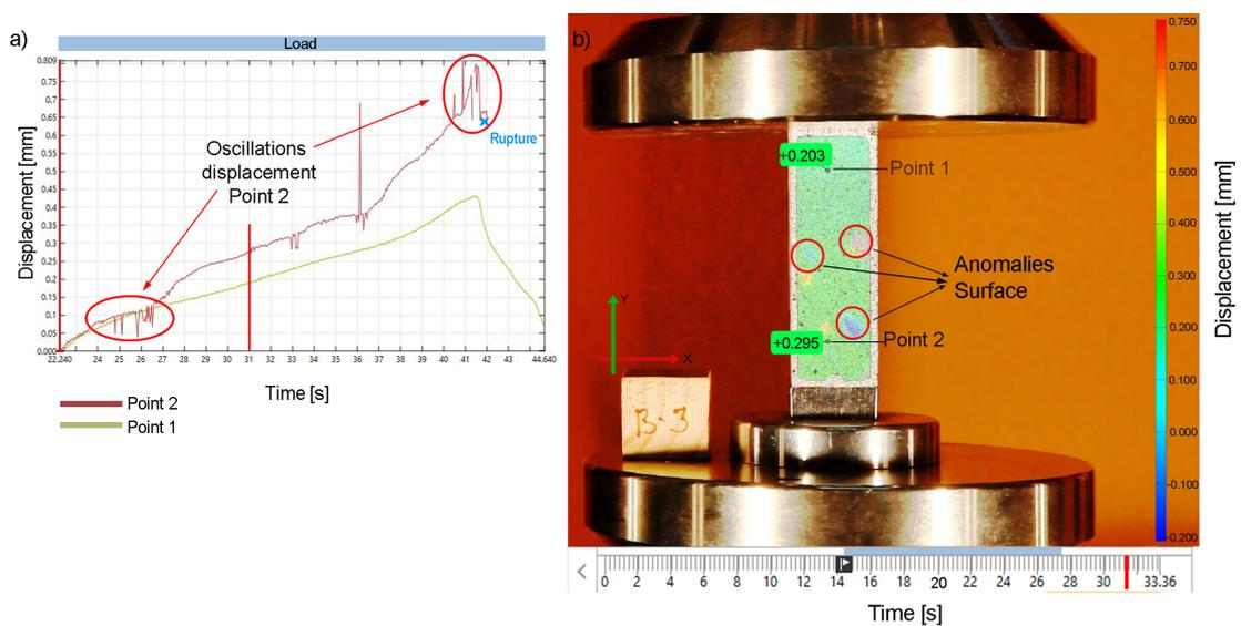
**Figure 11.** (a) Displacement diagram with oscillations of Point 2 ( $P_2$ ) and (b) anomalies of the displacements on the surface of specimen B3.
