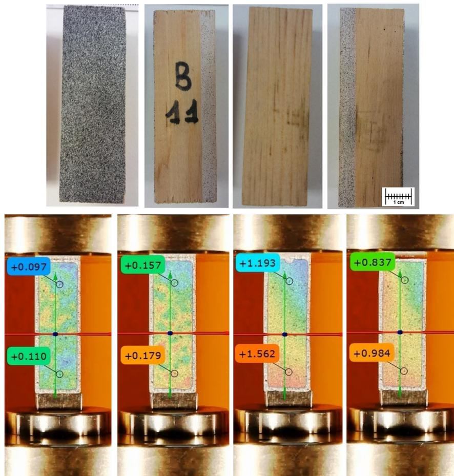
**Figure 22.** Final appearance of specimen B11 (all lateral faces). Frames of the test, in which the latter two show recovery in the elastic zone and separation from the press.
