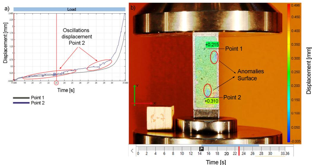
**Figure 12.** (a) Displacement diagram with oscillations of Point 2 ( $P_2$ ) and (b) anomalies of the displacements on the surface of specimen B7.
