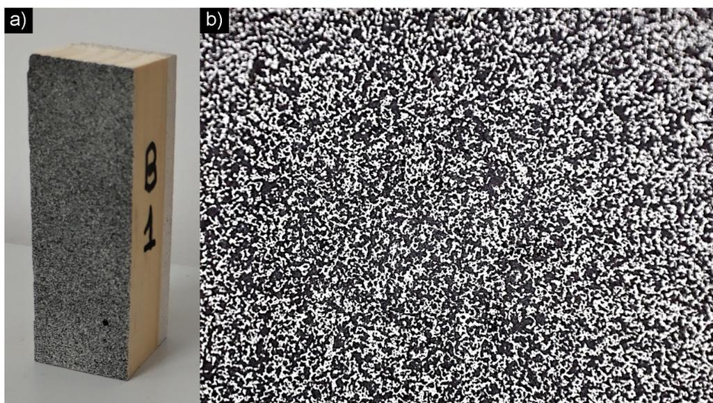
**Figure 2.** (a) Application of black speckled on a white base and (b) example of speckled pattern.
