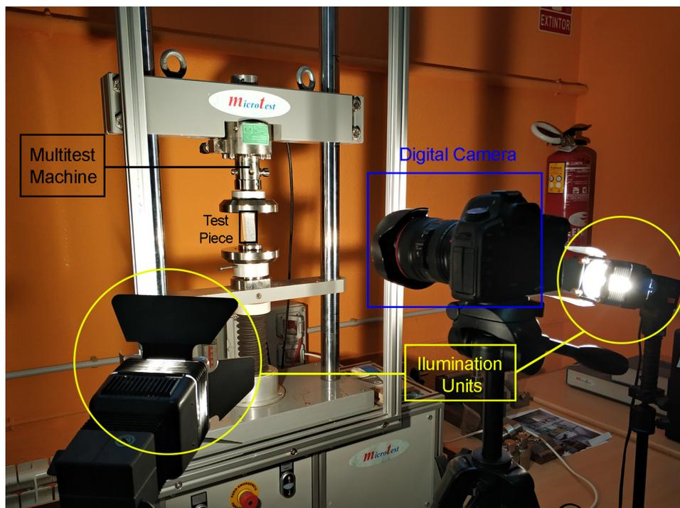
Figure 3. Complete test equipment.
