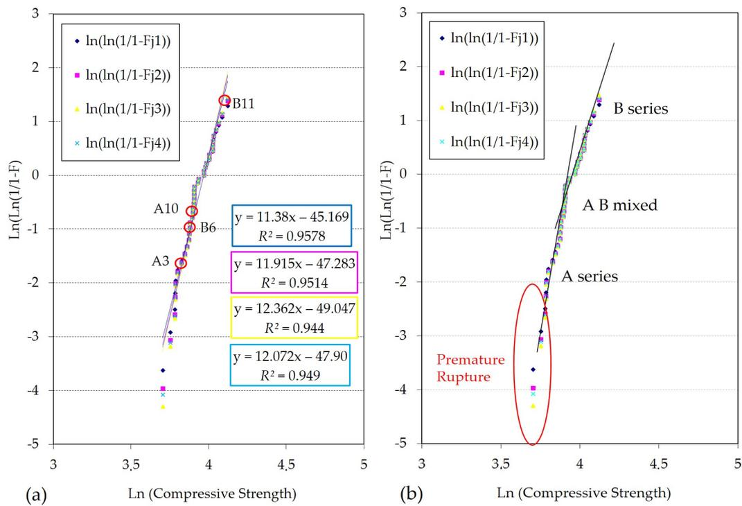
**Figure 15.** Weibull plot for all samples tested: (a) traceability of the selected specimens within the graph and (b) approximate discrimination of the series.
