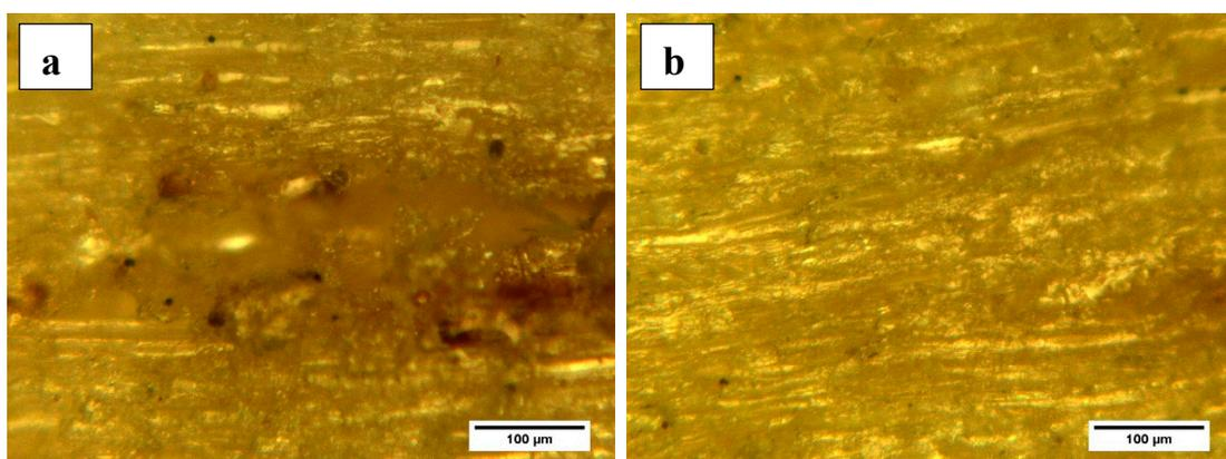
**Figure 17.** Microscopic appearance of the samples: (a) heterogeneity with associated porosity and (b) fiber arrangement.
