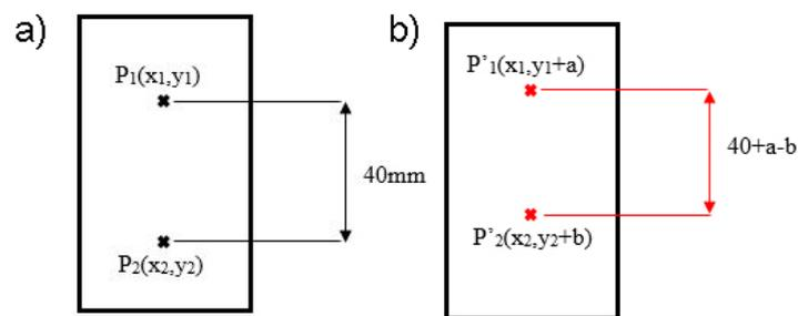
Figure 5. (a) Definition of points for the calculation of the strain and (b) displacement of the deformed points.
