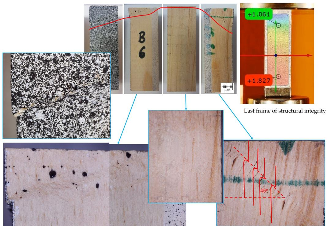
**Figure 21.** Appearance of the damage produced in the specimen B6. Comparison with the last frame of the structural integrity of the sample.
