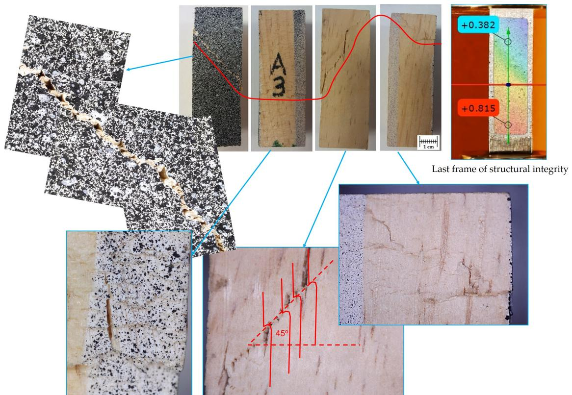
**Figure 19.** Appearance of the damage produced in the specimen A3. Comparison with the last frame of the structural integrity of the sample.
