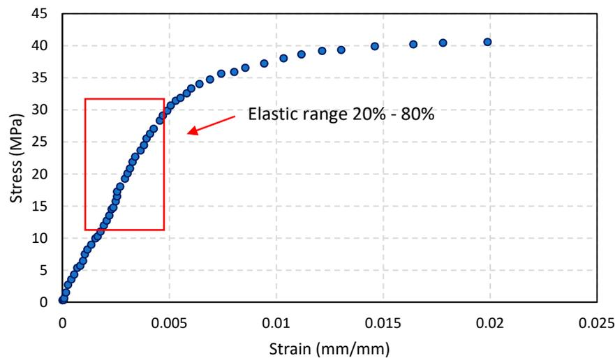
**Figure 8.** Area in which the modulus of elasticity in compression parallel to the grain ( $MOE_c$ ) is determined for specimen A1.
