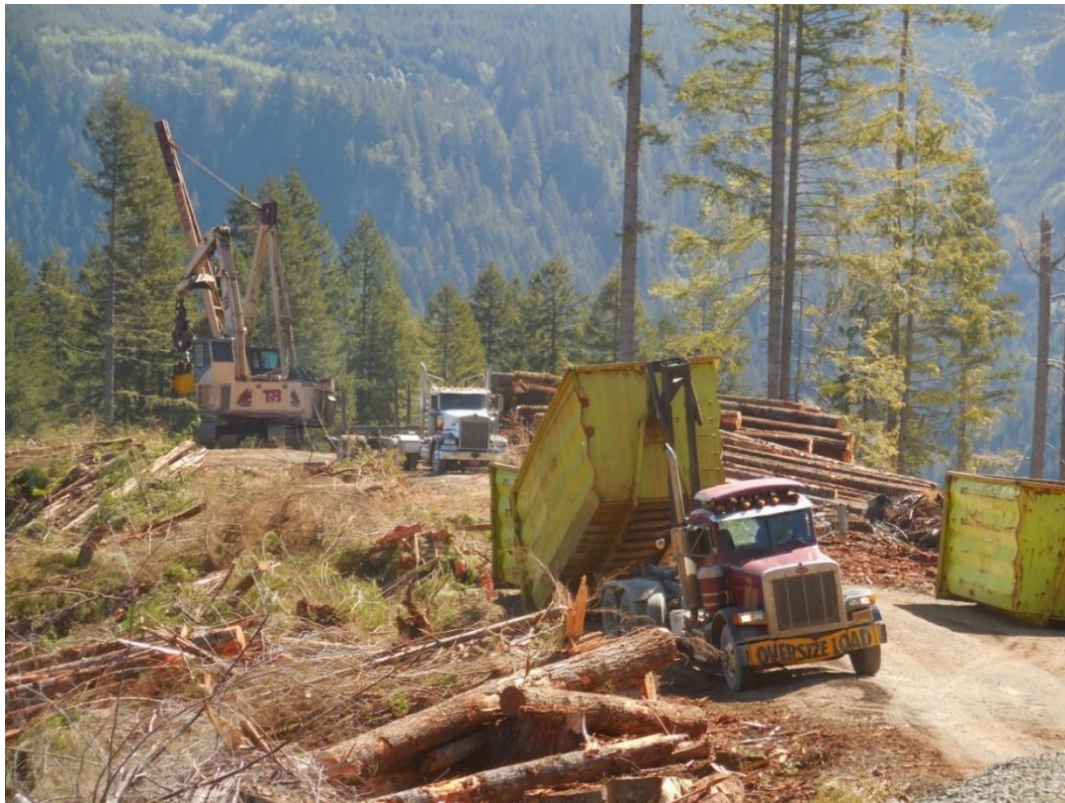
Figure 2. Skyline yarding and landing operational phases in the study comprised: (a) one yarder, (b) one loader, (c) one roll-off truck, (d) eleven roll-off containers, (e) two chasers, and (f) three choker setters.
