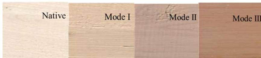
Figure 10. View of birch wood before and after heat treatment by individual modes.
